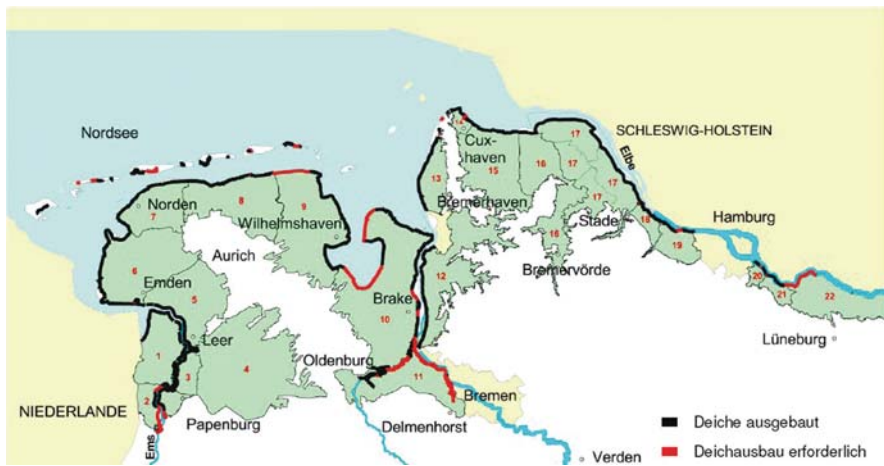
(a) Coastal stretches with insufficient safety condition
