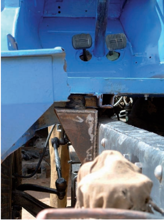
Photo 6.7 Reinforcing the cabin Source: K. Beck
