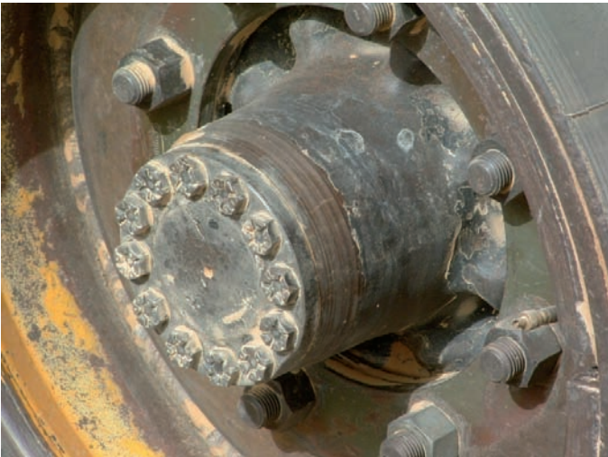
Photo 6.8 Wheel connected with bolts Source: K. Beck
