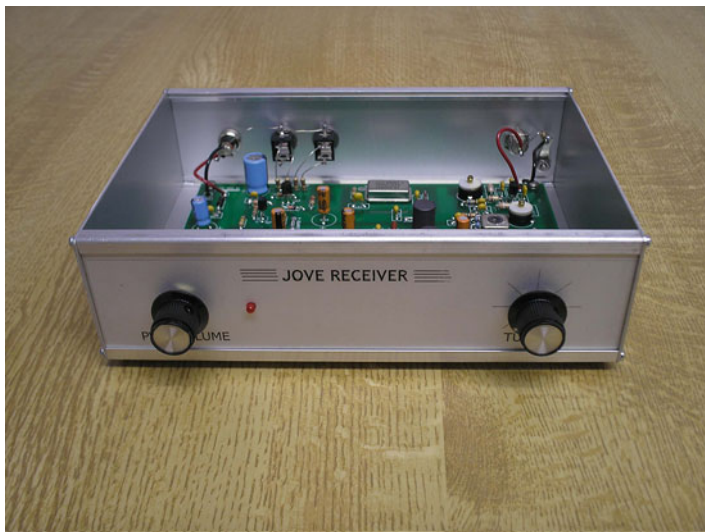
Fig. 7.3 The circuit board fitted into its enclosure after the final connections have been made and the temporary R32 (51 ohm) has been fitted
