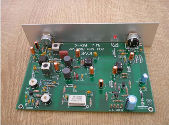
Fig. 7.2 Rear view of finished circuit board. (The crystal can be seen at the bottom center of the image)
