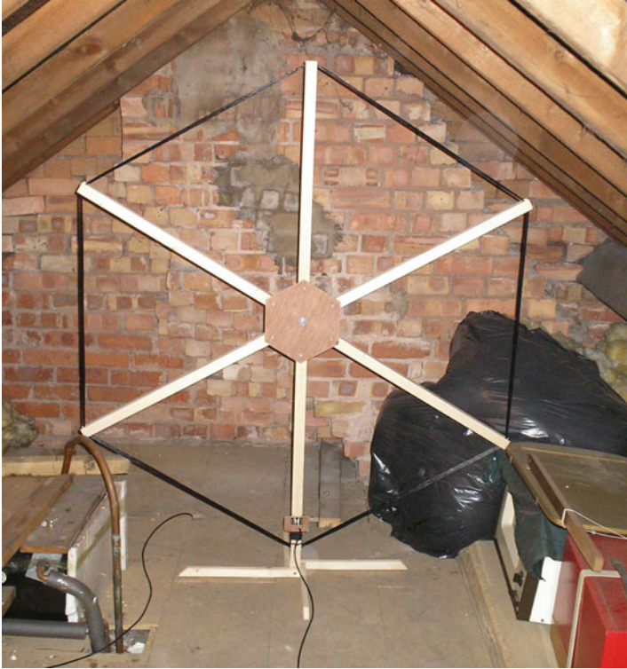
Fig. 5.5 Improved SuperSID antenna. Situated inside attic space
