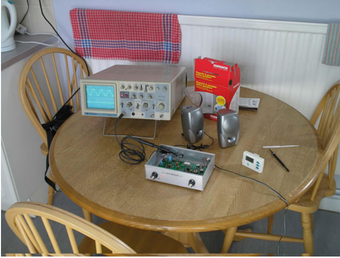
Fig. 7.4 Testing of the Radio Jove receiver. Using the oscilloscope method and externally powered speakers
