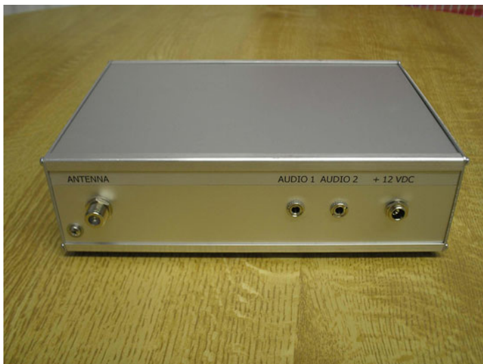
Fig. 7.6 The finished Radio Jove receiver rear view. Please note the connections, (from left to right) Antenna input, audio 1, audio 2 and 12 volt power input
