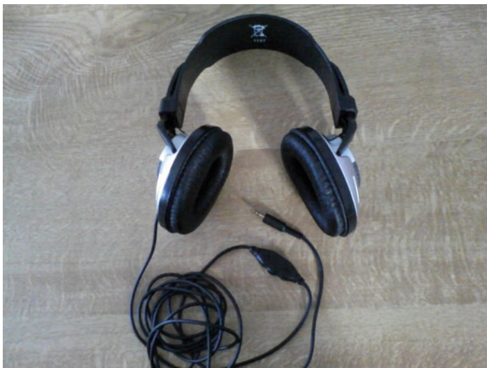
Fig. 4.8 The above image is of a full size pair of light weight headphones with good soundproofing cushions that fits all the way around the ears. There is also an inline volume control. This pair was not expensive to purchase. They are made mostly of plastic, but have soft leather ear cushions and deliver excellent sound quality
