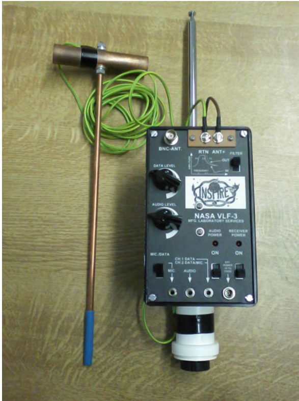
Fig. 6.4 The INSPIRE receiver showing antenna and copper ground stake on the left
