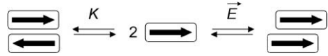
FIGURE 13.29. Illustration of the dimerization of chromophores and the influence of an applied electrical field.
