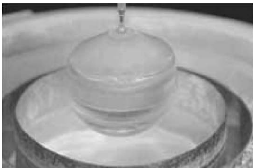
FIGURE 5.2. Near-stoichiometric LT single crystal of 3 inches diameter grown by the double crucible CZ method.
