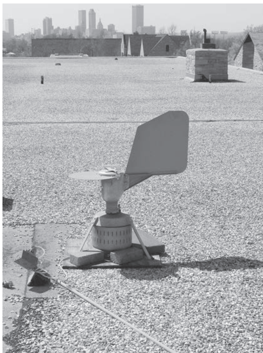
Figure 3-2. Burkard spore trap volumetric air sampler. (Courtesy Estelle Levetin, University of Tulsa.)
