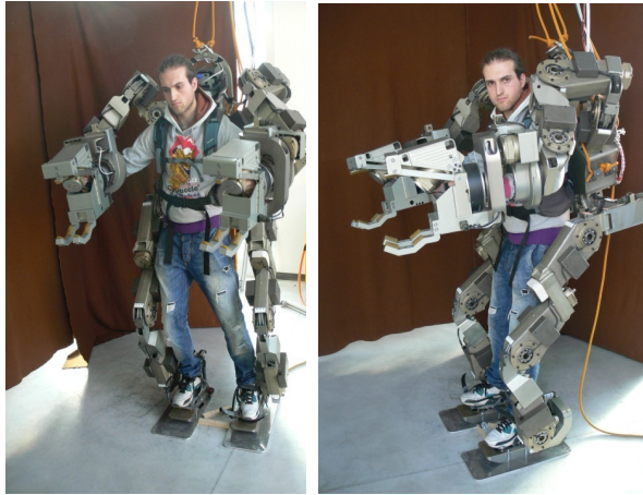
Fig. 20. Validation of the collaborative control with tests providing the physical interaction with a human wearing the BE during lateral motions (left) and longitudinal motions (right)
