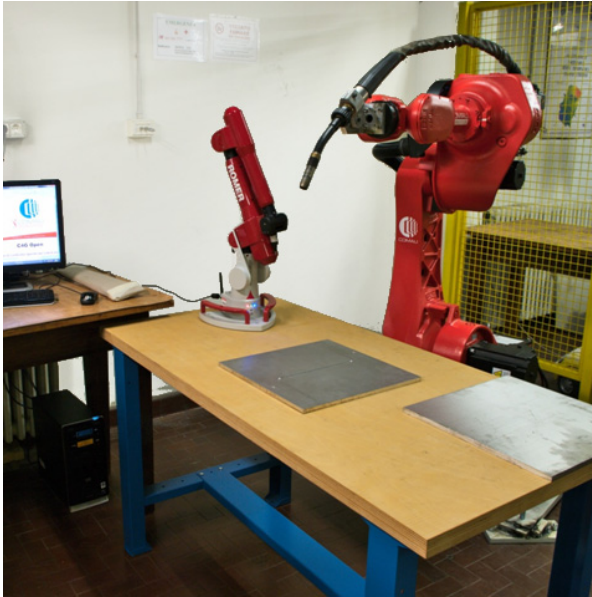
Fig. 9. Robot and CMM in the experimental area. There is a benchmark plate with a Z-shaped groove on the desk.
