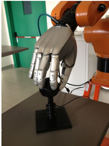
Fig. 12. The DLR-HIT II hand grasping the instrumented object in the sphere configuration
