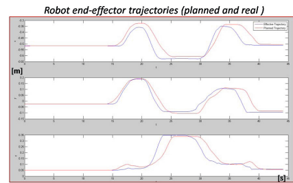
Fig. 14. Time course of real robot end-effector trajectory (blue line) and planned trajectory (red line) for K = 100 N/m
