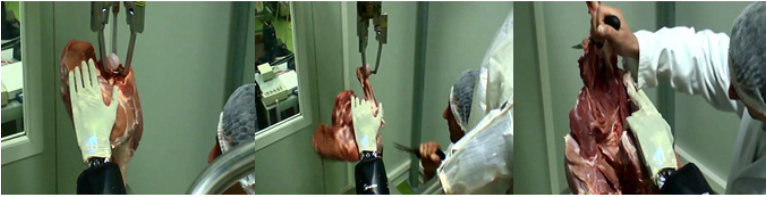
(b) Shadow hand integrated with an ABB robot arm at ADIV in France
