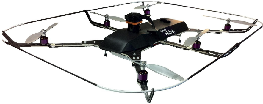
Fig. 6. The Flybox hexacopter by Skybotix equipped with a Hokuyo UTM-30LN laser scanner. A mirror, mounted on top of the laser, is used to deflect some rays towards the ground for altitude estimation. The low-level autopilot and the high-level computer are inside the housing.
