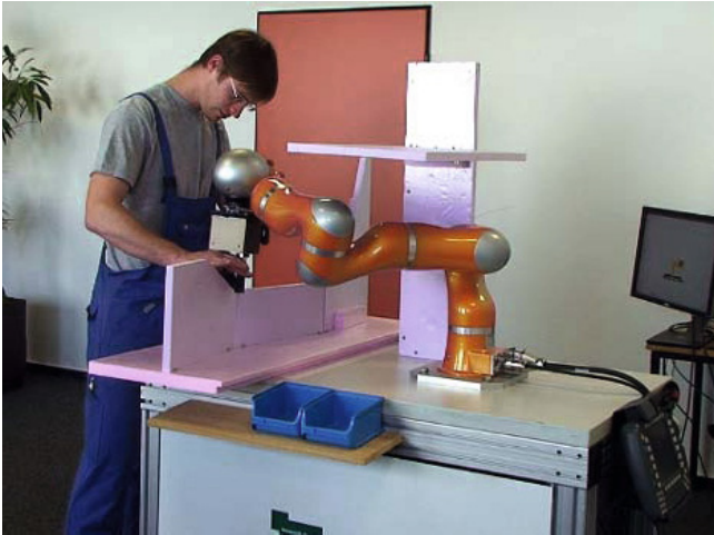
Fig. 1. A worker teaches a 3-D trajectory in a confined workspace while already being assisted by the robot's control system to avoid static obstacles in the scene [18]
