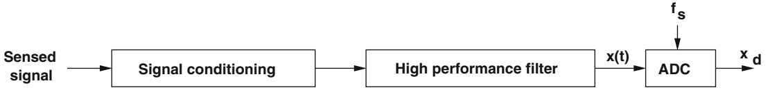
Figure 9.1: Analog signal sensing in embedded systems.
