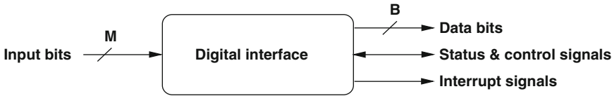
Figure 1.4: Digital input interfaces in embedded systems.
