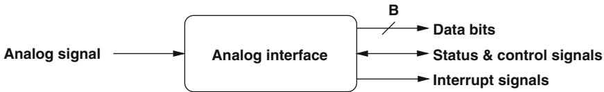
Figure 1.3: Analog input interfaces in embedded systems.
