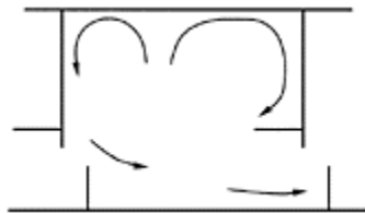
Figure 4. Flow pattern of the horizontal velocity field in planes located between 5cm above the bottom of the pool and the upper border of the sill.
