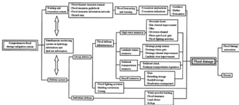
Figure 1. Comprehensive flood damage mitigation system.
