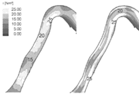
Figure 5. Influence of the ripples: computed shear stresses for removed ripple roughness (left) and with ripples at the flood plains (right) at km 1 +750 .
