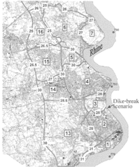
Figure 5. Detail of the polder area partitioned into compartments. Labels on the lines indicate the required heights. Compartments are numbered from 1 to 19.
