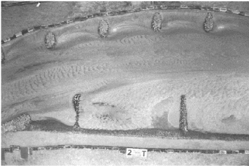
Figure 7. Control groynes at the inner bank to direct the flow to the outer bank and bank protection of the outer bank (final state of the measures).
