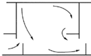
Figure 3. Flow pattern of the horizontal velocity field in a plane situated at 5cm above the bottom of the pool.
