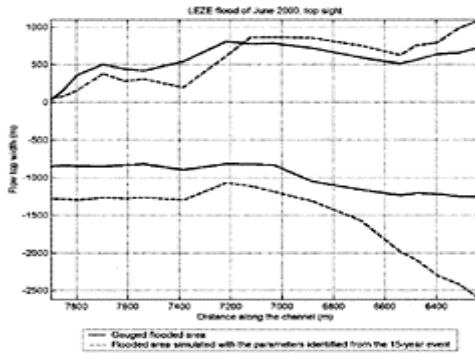
Figure 8. Comparison between gauged and simulated flow top widths for the flood of June 2000.
