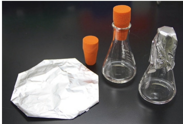
Fig. 1 Preparation of MS medium for cell culture. From left: double layer of aluminum foil, silicon cap, 100 mL flask capped with a silicon cap, 100 mL flask with a double layer of aluminum foil over the silicon cap
