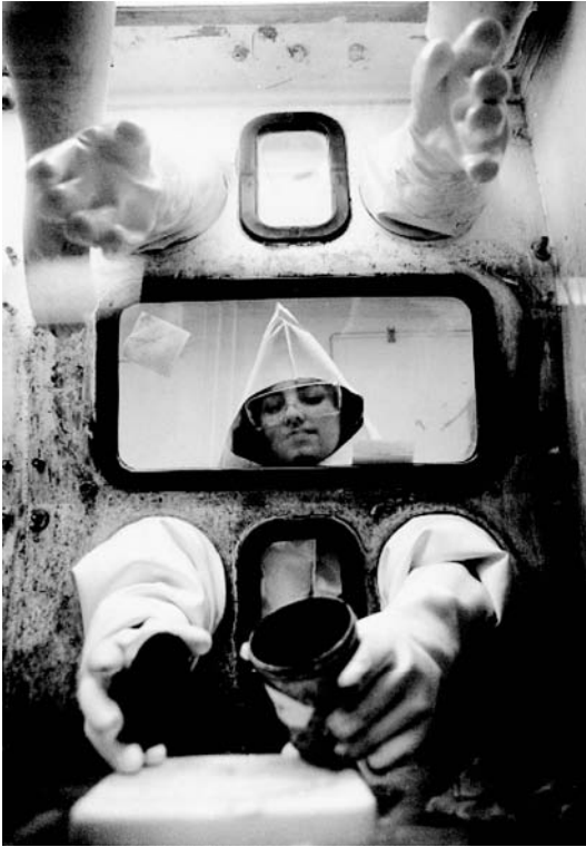
FIGURE 3.17 Plutonium-handling glove box. (From U.S. Department of Energy, Linking Legacies Connecting the Cold War Nuclear Weapons Production Processes to Their Environmental Consequences , DOE/EM-0319, Office of Environmental Management, Washington, DC, Jan. 1997; http://legacystory.apps.em.doe.gov ; accessed 8/5/04.)
