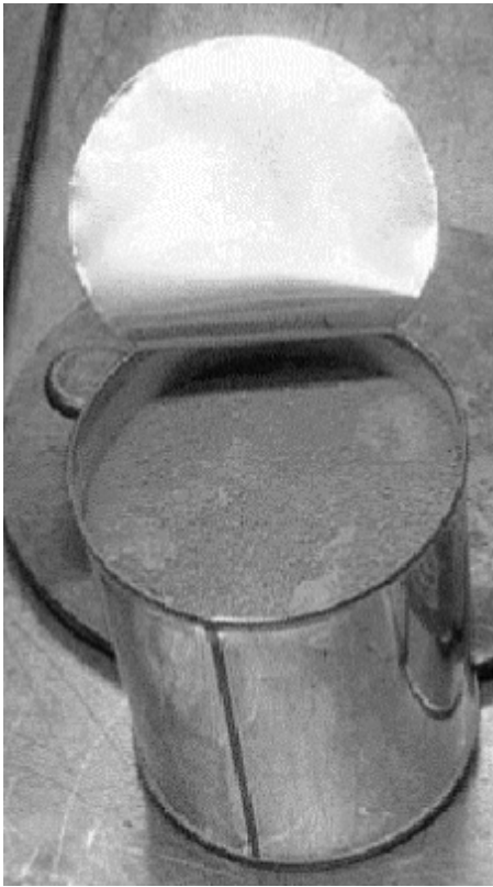
FIGURE 3.19 Plutonium oxide. (From U.S. Department of Energy, Linking Legacies Connecting the Cold War Nuclear Weapons Production Processes to Their Environmental Consequences, DOE/EM-0319, Office of Environmental Management, Washington, DC, Jan. 1997; http://legacystory.apps.em.doe.gov ; accessed 8/5/04.)
