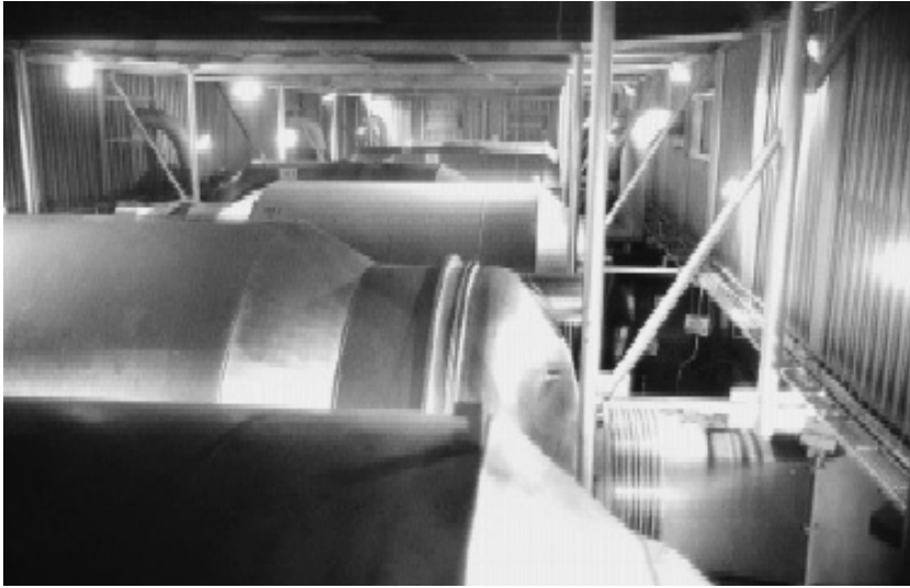
Figure A3.4 Gaseous diffusion stage of a U.S. enrichment facility. (From U.S. Department of Energy, Linking Legacies Connecting the Cold War Nuclear Weapons Production Processes to Their Environmental Consequences , DOE/EM-0319, Office of Environmental Management, Washington, DC, Jan. 1997; http://legacystory.apps.em.doe.gov ; accessed 8/5/04.)
