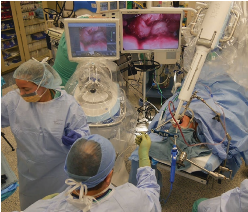
Fig. 19.6 Surgeon placing compatible Flex® Instruments into side channels of positioned flexible robotic scope
