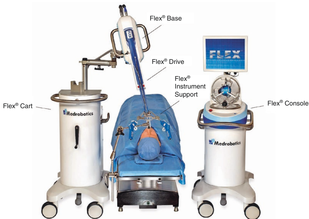
Fig. 19.1 Components of the Flex® Robotic System
