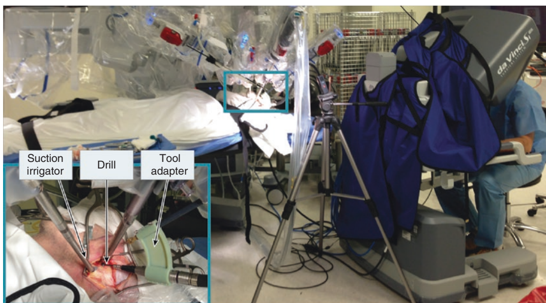
Fig. 17.3 Operating room with the da Vinci Si for otologic surgery. Inset is a close-up of the initial position of the endoscope, suction/irrigator, and drill attached with the custom tool adapter (With permission) [21]
