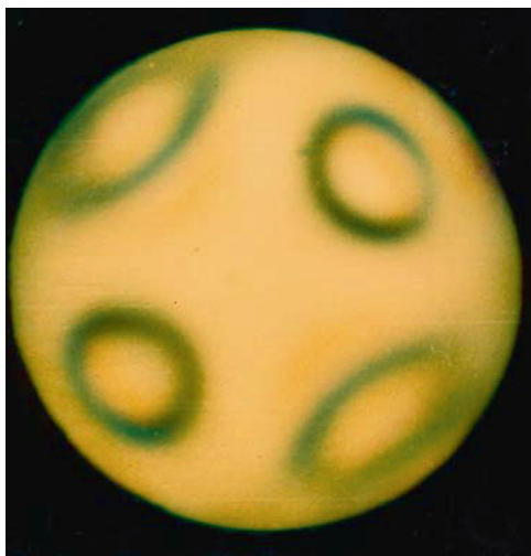
Figure 4.15. Example of an interference figure for heterogeneous potassium ferrocyanide trihydrate crystal
