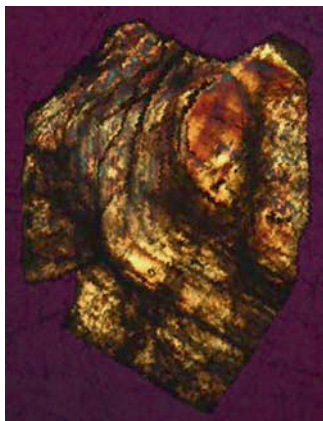
Figure 2.33. Anomalous birefringence in (0001) section of beryl, schematically shown in Figure 2.34. Birefringence changes at zone boundaries and cracks are visible
