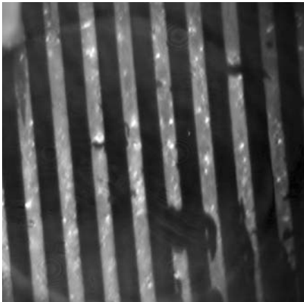
Fig. 14.48. Interferometric microscope image of protein grating, image width 65microns
