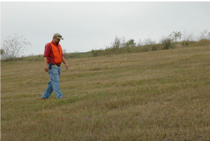
Fig. 15.4 Inspecting a landfill slope for side seeps
