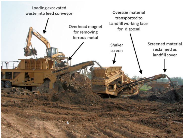
Fig. 17.12 Processing mined landfill material utilizing a shaker screen and overhead drum magnet
