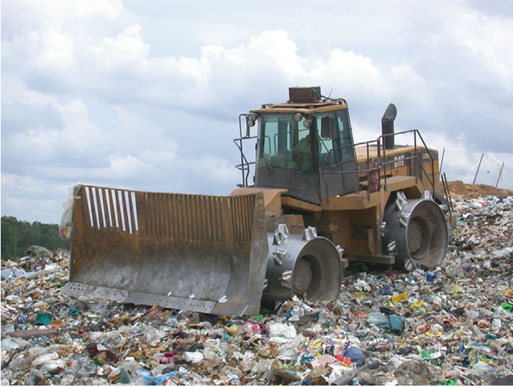
Fig. 1.5 Waste compaction in organized cells is a fundamental component of sanitary landfill operation
