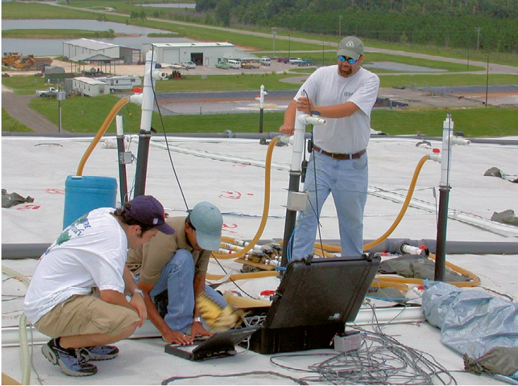
Fig. 4.17 Addition of liquids into a vertical well cluster at NRRL and measurement of flow rates and liquid depths
