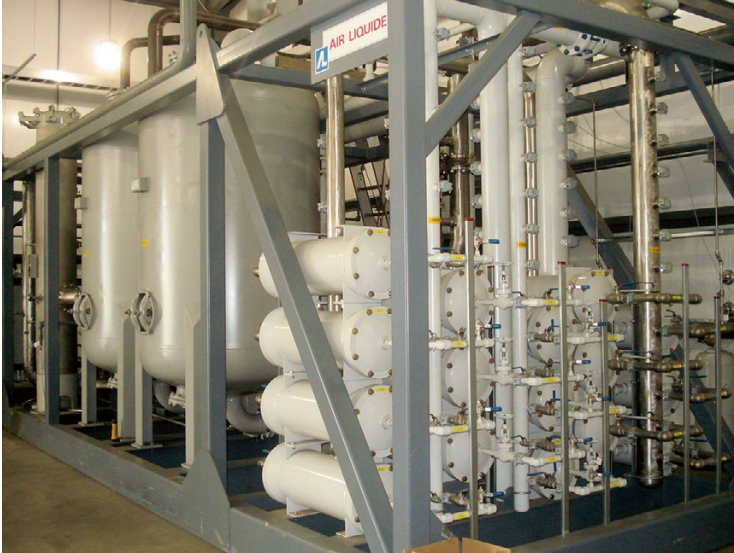
Fig. 19.3 Pressure swing adsorption and membrane equipment for cleaning up landfill gas to high energy content
