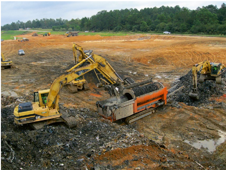
Fig. 1.10 Landfill mining allows reclamation of metals, soil, and degraded organic matter
