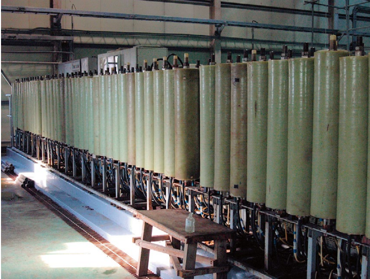
Fig. 11.18 A bank of spiral wound reverse osmosis membranes used as a polishing step in an integrated leachate treatment operation
