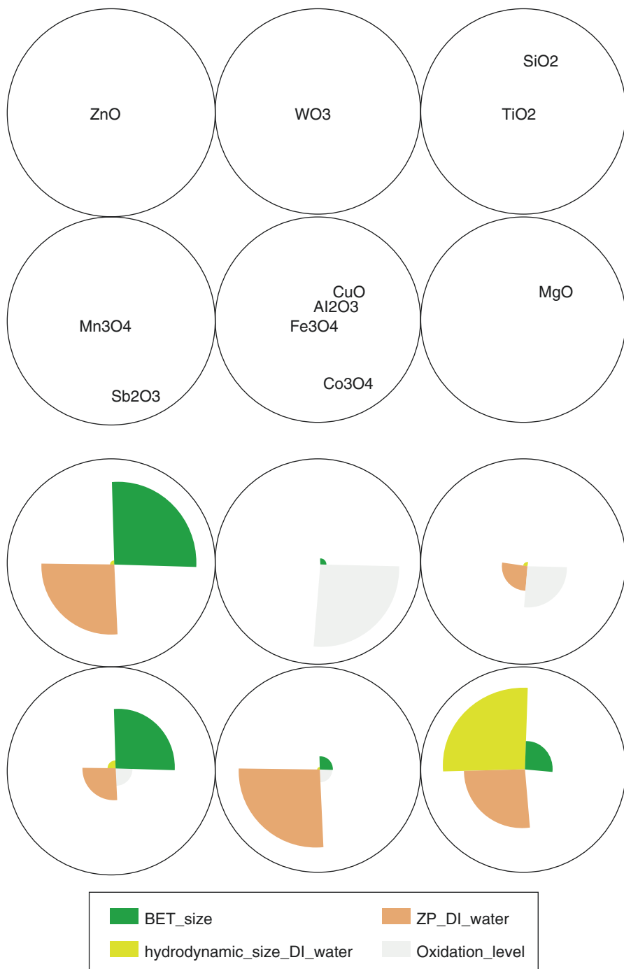
Fig. 9.10 Self-Organizing Map (SOM) clustering of metal oxide nanoparticles in MODERN's library. Clustering was performed based on the group of physicochemical properties reported in Table 9.5. (Top) Identification of eNPs in each category. (Bottom) Physicochemical property profile of each category
