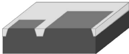
(c) Vapour phase chemical deposition of an oxide in the trenches, then leveling by mechanochemical polishing
