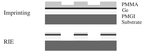
Fig. 6.3. Three-layer nanoimprint process invented to obtain high aspect ratios. Fabrication consists in imprinting the upper layer (PMMA), then transferring imprinted features by RIE to the relatively thick underlying resist layer (in this case, PMGI), which is heat stable at the imprint temperature, via a thin intermediate metal film (here, Ge)
