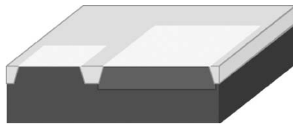
(f) Thermal oxidation of Si to obtain the gate insulator SiO_2
