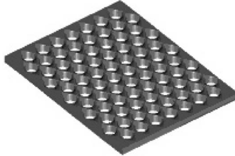
Fig. 16.24. Illustration of a membrane-type 2D photonic crystal, consisting of holes in a dielectric surrounded by air both above and below
