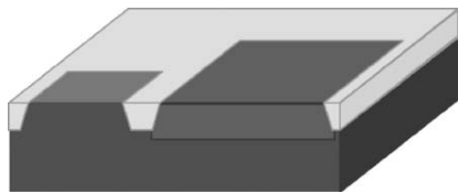
(e) Post-implantation anneal to remove defects induced by ion bombardment in the crystal structure and electrically activate the dopants by placing them at substitutional sites. During the anneal, impurities diffuse throughout the substrate
