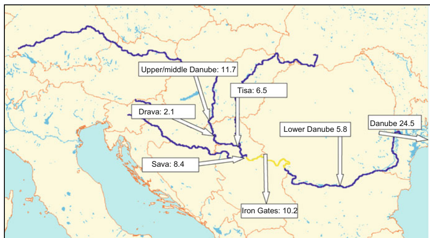
Fig. 7 Estimated total phosphorus in-stream loads (kt/year) of the Danube River (based on data from 1997 to 2001)
