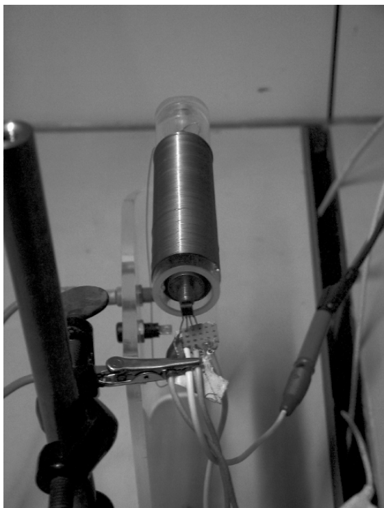
Figure 4. Setup of the remote experiment on hysteresis, the magnetic coil in the middle, Hall probe in front
