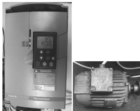
Fig. 10. ALTIVAR 58 inverter and the AC machine
