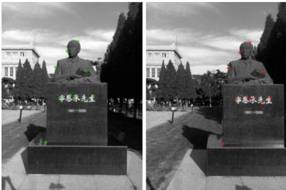
Fig. 29.7 Matching result of the correcting algorithm based on spatial distribution descriptor
