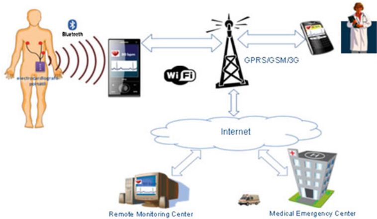
Fig. 28.1 Block diagram of the system for heart monitoring on mobile device
