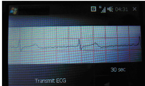
Fig. 5. Measured one-lead ECG signals on ECG smartphone
