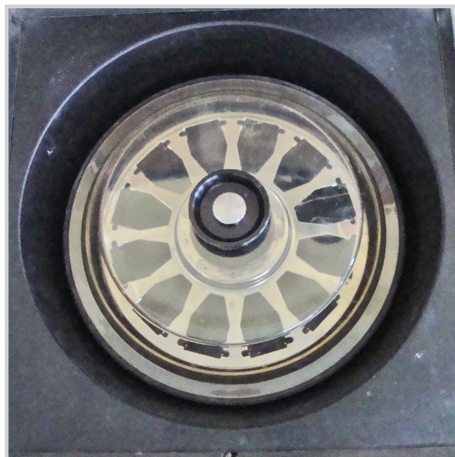
Fig. 16.7: Interior chamber of the cytocentrifuge machine
