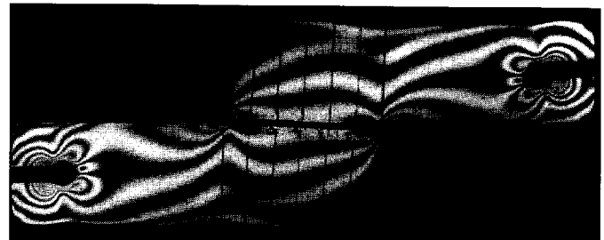
Fig 7. Photoelastic test on single lap joint
