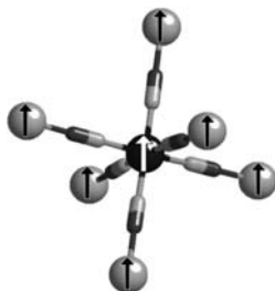
Fig. 10.2 Schematic view of the magnetic core of the heptanuclear cluster of formula [\text{Cr}^{\text{III}}(\text{CN-Ni}^{\text{II}}\text{-L})_6]^{9+} , with the ferromagnetic alignment of the spin indicated by the arrows. The cyanide bridges are shown as rods, with the carbon atom in pale grey
