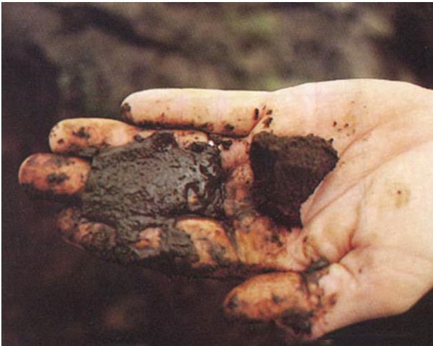
Fig. 7.8 The noncohesive thixotropic nature and extremely high liquid limit of the Andosols is demonstrated by a clod of soil, and the same soil after applying some disturbance and pressure on the clod
