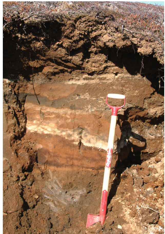
Fig. 12.6 Thick, coarse, rhyolitic Hekla layers in soil (yellowish). These layers lack cohesion and are very susceptible to wind erosion if exposed, causing damage to surrounding systems after erosion processes are initiated. Grains >2 mm in diameter are common and are easily moved by the wind
