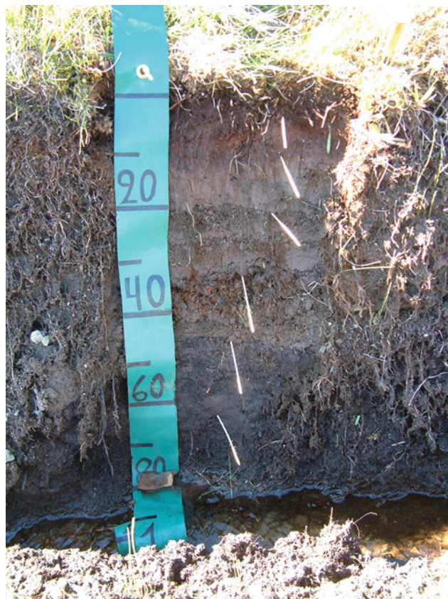
Fig. 6.12 Histosol from Dýrafjörður in the Westfjords. A newly dug ditch in a gently sloping wetland. All horizons are organic, the soil has low pH of about 4 and limited allophane content
