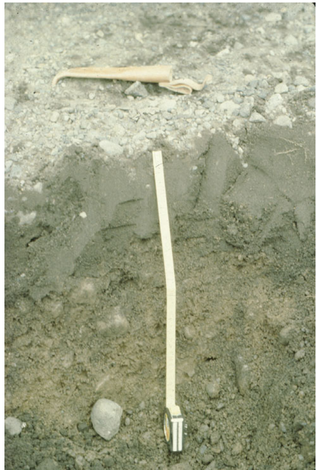
Fig. 7.19 The Sigalda Pedon (South highlands—Cambic Vitrisol) from Arnalds and Kimble (2001). The soil is sandy but some allophane and organic matter are found in the Bw horizon
