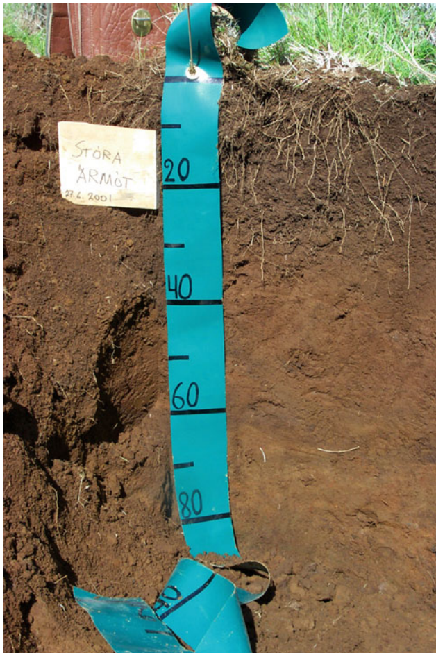
Fig. 5.2 A dark colored Andosol from the southern lowlands. Note, clear granular structure in the A horizons and roots extending deep into the soil. Carbon rich horizons reach for the entire depth of the soil as is common with Andosols
