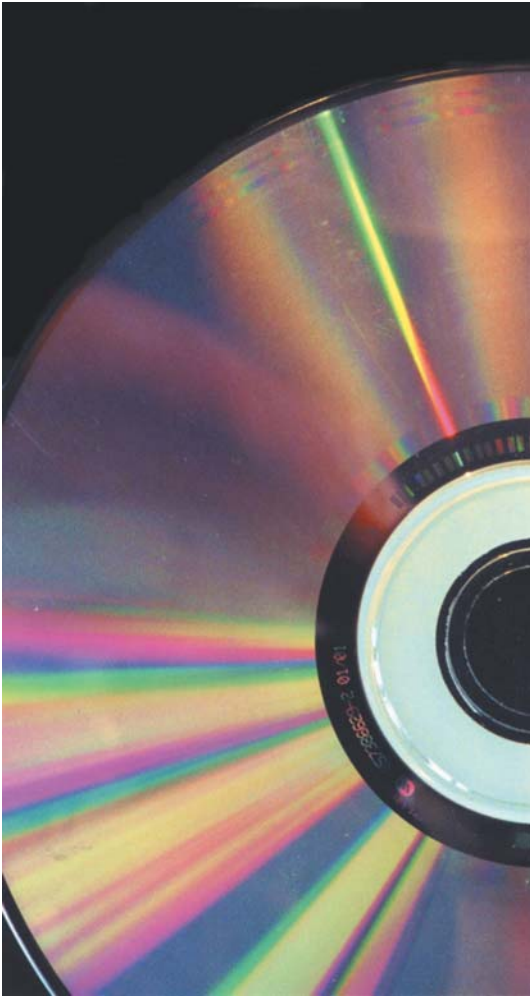
Figure 8.1. One of the most widespread examples of a grating; diffraction resulting from burning a compact disc.
