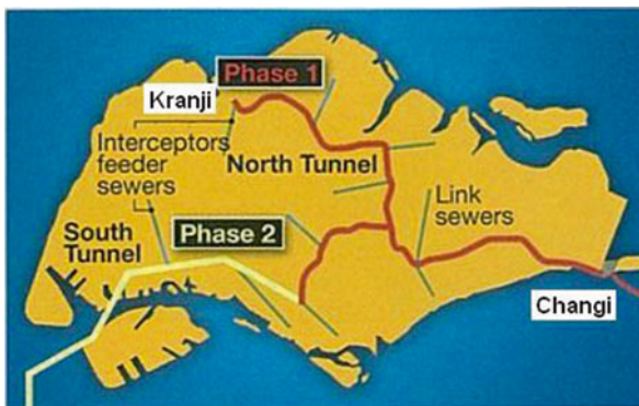
Fig. 26.2 Layout of Singapore's deep tunnel sewage system
