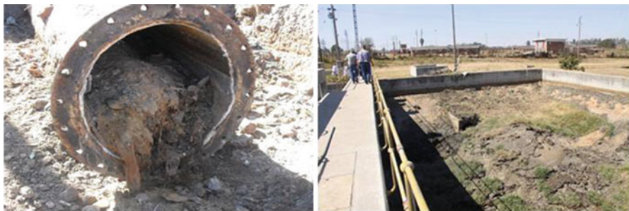
Fig. 4.2 High levels of sand in sewers ( left ) can cause downstream problems at sewage treatment plants ( right ) (Photographs: City of Harare)
