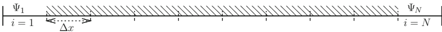
Fig. 4.1 One-dimensional grid. The TDSE is solved within the marked region on a number N_x discrete grid points. i = 1 and i = N_x are defined by the boundary conditions
