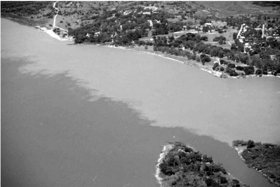
**Figure 5.6** Oblique aerial photograph of the junction of the Río Paraná and Río Paraguay. Note the contrast produced by the higher suspended sediment concentrations of the Río Paraguay and the vorticity present along the mixing interface. A colour reproduction of this figure can be seen in the colour section towards the centre of the book.
