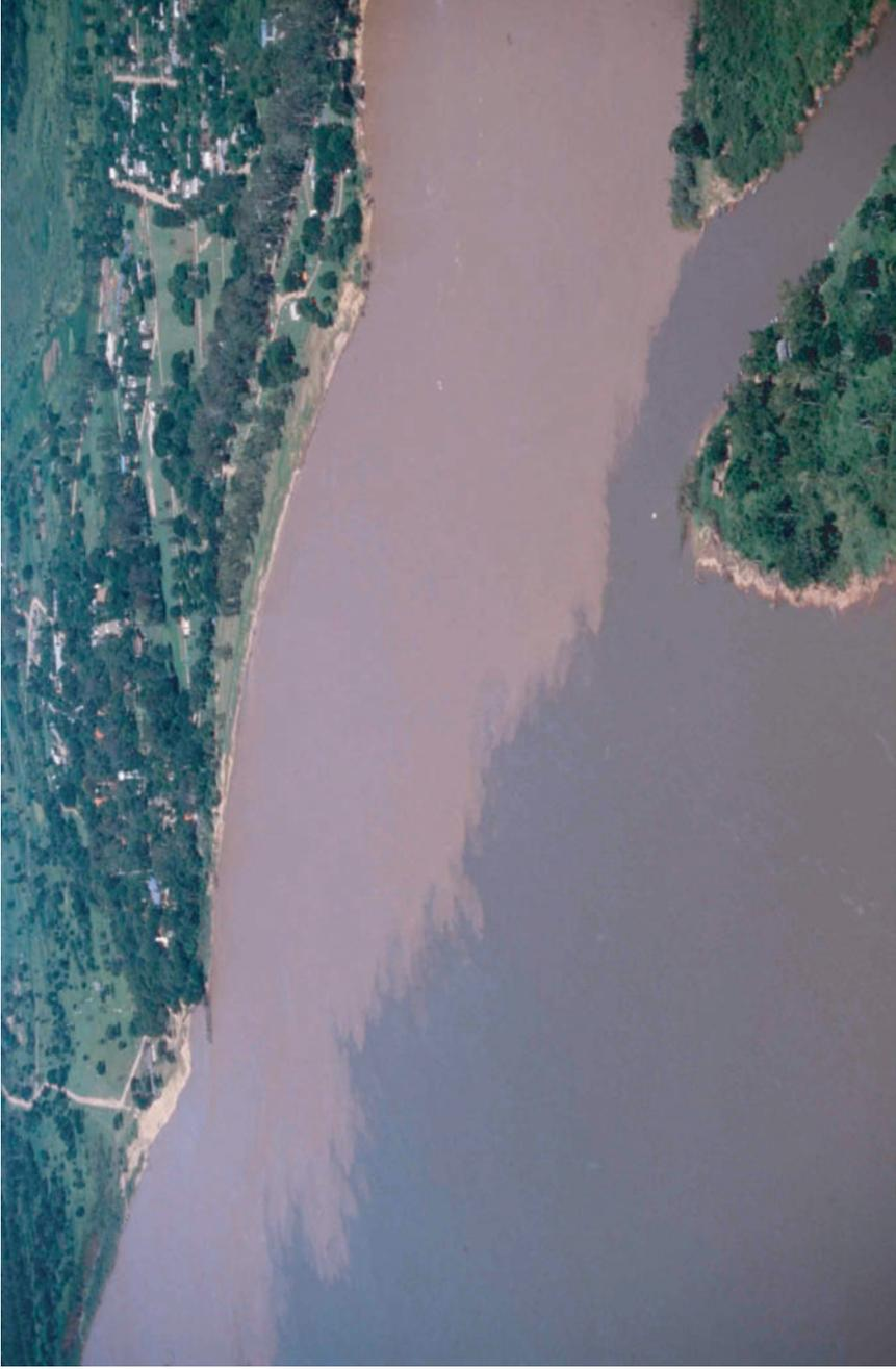
**Figure 5.6** Oblique aerial photograph of the junction of the Río Paraná and Río Paraguay. Note the contrast produced by the higher suspended sediment concentrations of the Río Paraguay and the vorticity present along the mixing interface.
