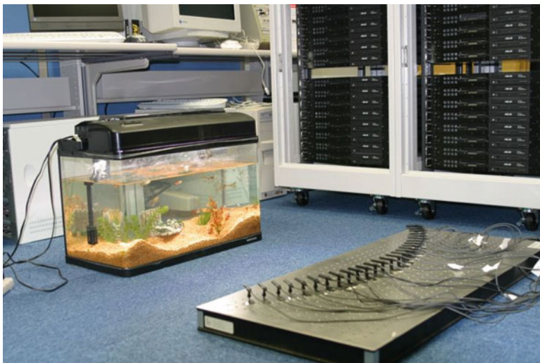
Fig. 9.2 One-dimensional arc capturing system of FTV
