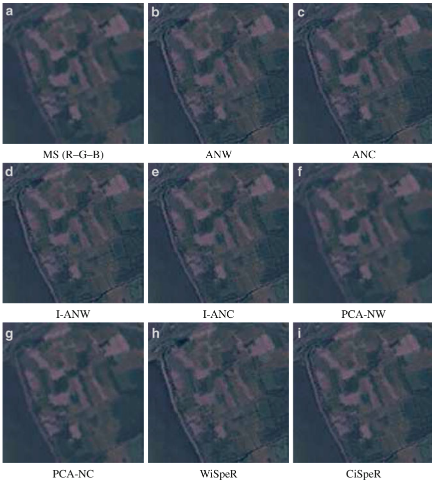
Fig. 20.3 (a) Low-resolution image formed from the R-G-B bands of the MS LandSat image. (b)–(i) Pansharpened images using the methods under study
