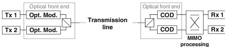
Fig. 8.1 Concept of PDM enabled by MIMO processing at the receiver, with Tx baseband transmitter, Opt. Mod. optical modulator, COD coherent optical detector, and Rx baseband receiver
