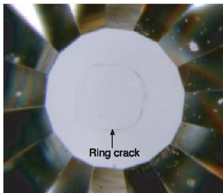
Figure 2. Photomicrograph showing indentation (ring crack) of diamond anvil by the high-pressure form of cold compressed graphite. (From Mao et al. , 2003; Reprinted with permission from AAAS).
