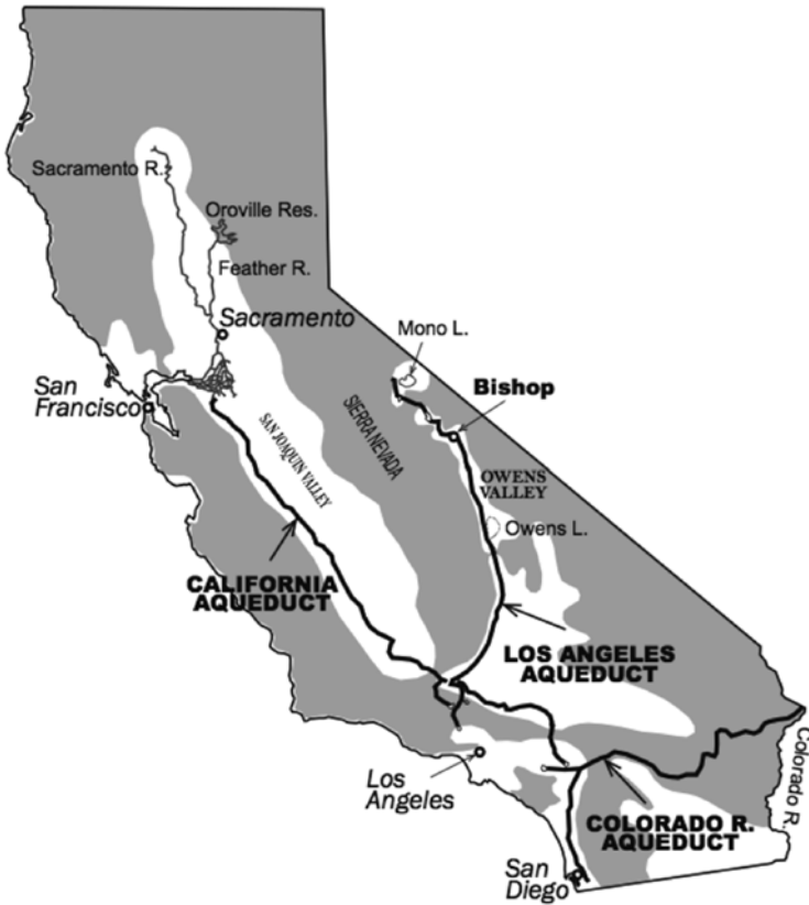
Fig. 4.23 The three major aqueducts that supply water to Los Angeles. These include the Los Angeles Aqueduct from the Owens Valley, the Colorado River Aqueduct from the Colorado River, and the California Aqueduct from Northern California (Map courtesy of Dr. Lynn Ingram, from Lynn Ingram and Frances Malamud-Roam. 2013. The West Without Water . University of California Press, Berkeley. 256 p. Used by Permission University of California Press)
