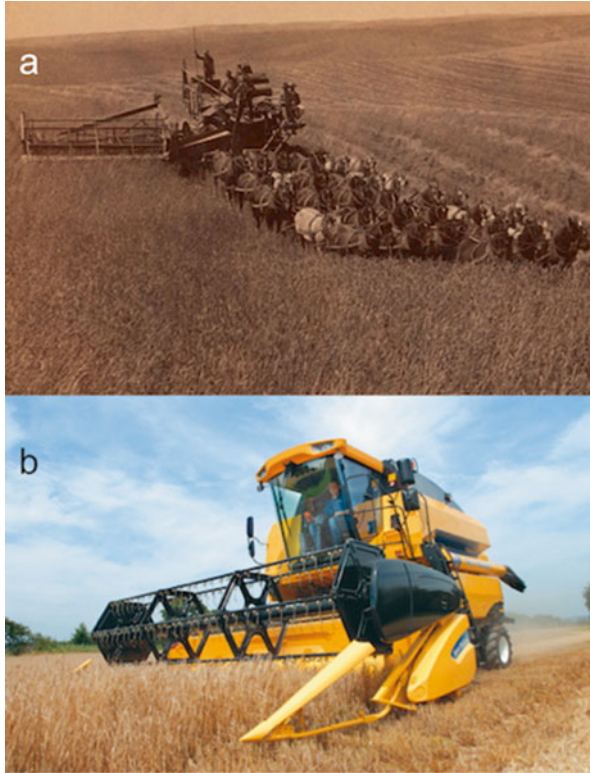
Fig. 8.6 Farming on the American plains. (a) 33 horsepower (HP) controlled by five workers. (b) 200 HP combine controlled by one worker (Images courtesy of Mario Giampetro)
