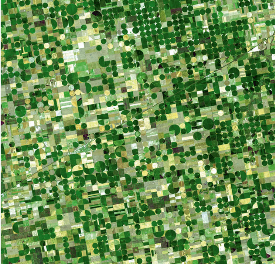
Fig. 5.2 Center Pivot Irrigation Systems in Kansas. Water is pumped from the Ogallala Aquifer to irrigate these crops. (By NASA [Public domain], via Wikimedia Commons)
