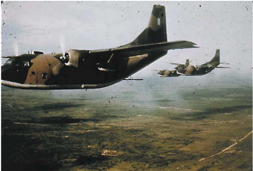
Fig. 3.6 The UC-123 K "Provider" with its Modular Internal Spray System was the "work-horse" for RANCH HAND. This high-wing, twin-engine assault transport had excellent low speed maneuverability, and the high-mounted wings allowed convenient positioning of wing spray booms. Note the spray boom mounted aft of the cargo door and near the tail of the aircraft (Photograph courtesy of J. Ray Frank, Frederick, Maryland)
