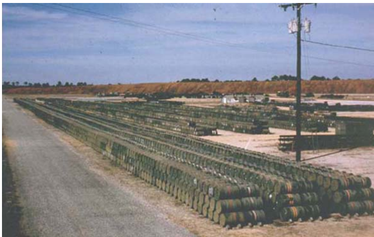
Fig. 4.22 Photograph of the Agent Orange inventory in 1974, at the Naval Construction Battalion Center; the inventory was initially stored upright on pallets, but the drums were subsequently placed on their sides on wooden dunnage (Photograph courtesy of AFLC, Kelly AFB, Texas)
