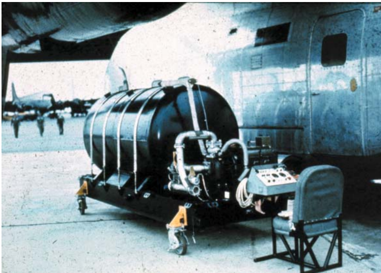
Fig. 3.5 USAF photograph of the A/A 45Y-1 Internal Defoliant Dispenser (Photo courtesy of the Air Force Armament Laboratory, Eglin AFB, Florida)
