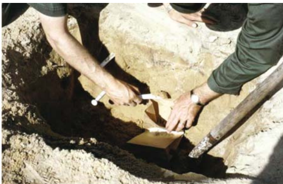
Fig. 6.42 Two AFATL scientists collecting 15-centimeter soil samples to a depth of 90 centimeters from Grid 1 for analysis of TCDD in June 1973, Test Area C-52A, Eglin AFB, Florida (Photograph courtesy of A.L. Young)
