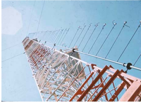
Fig. 6.5 The 90-m tower in the center of Test Area C-52A used for collecting dispersion and wind data in support of Spray Equipment Test and Evaluation Missions, Eglin AFB, Florida, 1969 (Photograph courtesy of A.L. Young)
