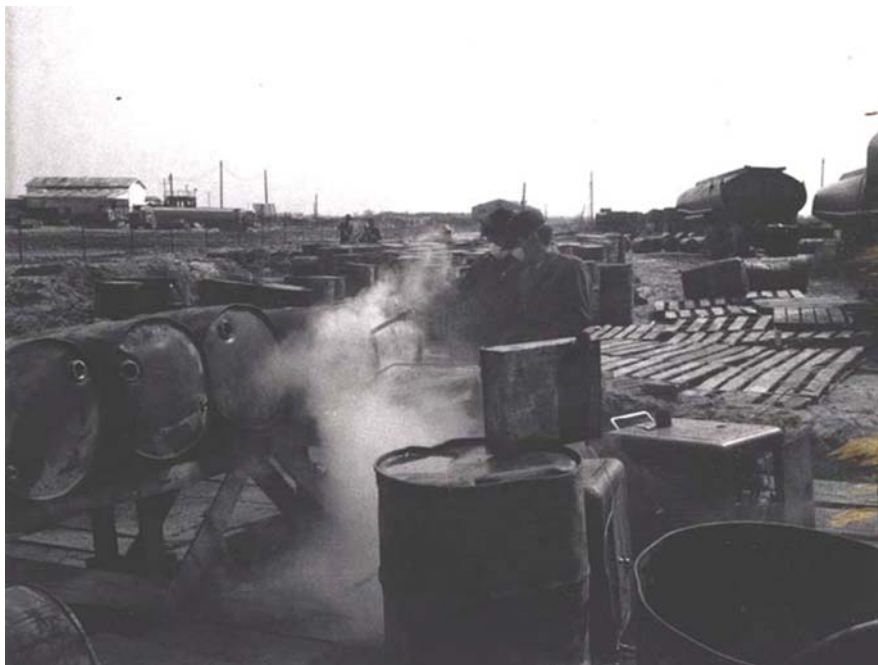
Fig. 4.10 Usable empty Agent Orange drums were steam cleaned and provided to the Vietnamese Air Force (VNAF), Operation PACER IVY, Da Nang Air Field, 15 January 1972 (Carmichael Journal 1972)
