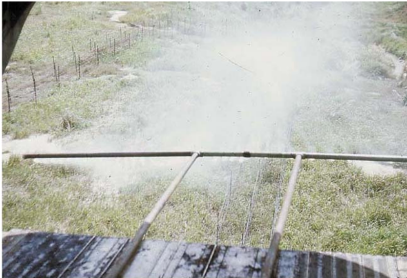
Fig. 3.22 A photograph of the base perimeter of Phan Rang Air Base at the time of aerial application of Agent Blue by the use of a modified spray rig mounted in the cargo bay and door of a C-7. Notice the “in-depth” wire fencing (i.e., two rows consisting of three lines of fence, each 1 m apart). Because the base bordered civilian dwellings, this fence arrangement was intended to keep civilians from inadvertently entering base perimeter areas (photograph courtesy of US Army Chemical Corps)
