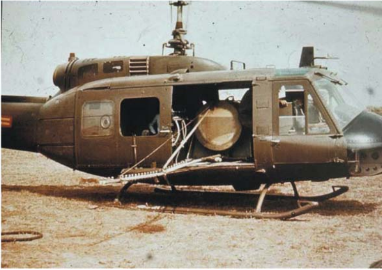
Fig. 3.7 The Military UH-1 series of helicopters generally sprayed the herbicides. The most common spray systems were the HIDAL and AGRINAUTICS units. They could be removed from the aircraft in a matter of minutes. Each unit consisted of a 760-l tank and a collapsible 9.8-m spray boom (Photograph courtesy of the US Army Chemical Corps)
