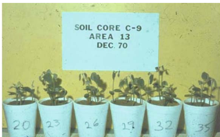
Fig. 6.21 Soybean bioassay of a 90-cm soil core from Site C-9 divided into 15-cm increments showing negligible levels of herbicide residue, December 1970, Test Area C-52A, Eglin AFB, Florida (Young 1974)
