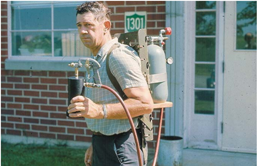
Fig. 2.3 A 1970 photograph of the hand applicator used in the initial defoliant screening tests at Fort Detrick. The sprayer was a specially calibrated unit capable of delivery less than 0.1 kg/ha of candidate defoliant (photograph courtesy of A. Young)
