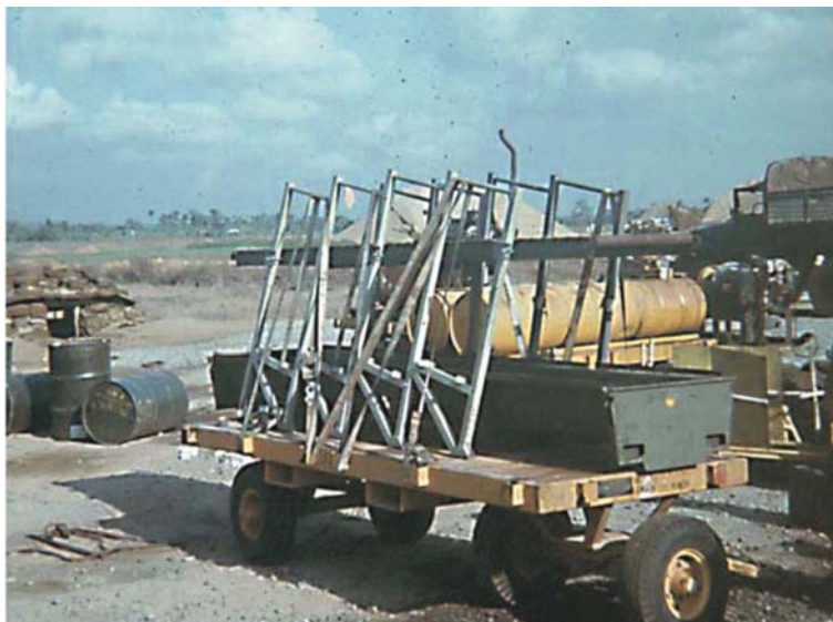
Fig. 3.15 At each of the RANCH HAND Bases trailer mounted drain racks were used to recover the remaining “dregs” of herbicide from the 208-l drums. These dregs were used for perimeter vegetation control (Photograph courtesy of J. Ray Frank, Frederick, Maryland)
