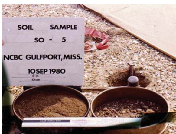
Fig. 7.17 A photograph taken 10 September 1980 by personnel from the Engineering Services Laboratory showing the sampling protocol for collecting soil samples on the former Herbicide Orange Storage Site, NCBC (Photograph courtesy of Air Force Engineering and Services Laboratory, Tyndall AFB, Florida)
