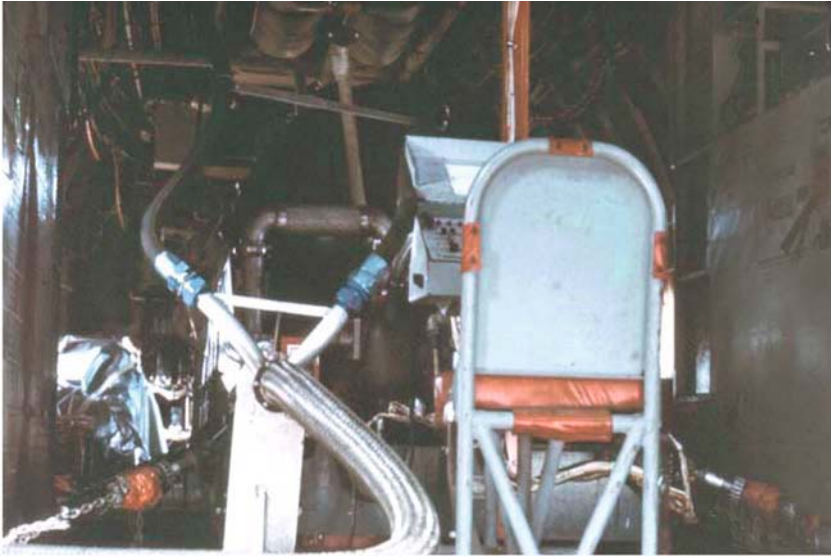
Fig. 6.10 An interior view of the A/A 45 Y-1 Internal Modular Spray System mounted in the UC-123 K aircraft, Hardstand 7, Eglin AFB, Florida 1969 (Photograph courtesy of AFATL, Eglin AFB, Florida)
