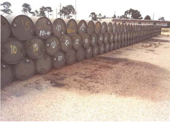
Fig. 7.5 A photograph taken at NCBC on June 1975 showing the soil contamination initiated by a “pinhole” size leak in a drum of Agent Orange identified by an Analysis Sequence Number 10 (ASN 10), as a product produced by The Dow Chemical Company, and found to have a TCDD mean concentration of 0.25 ppm (Photograph courtesy of AFLC, Kelly AFB, Texas)
