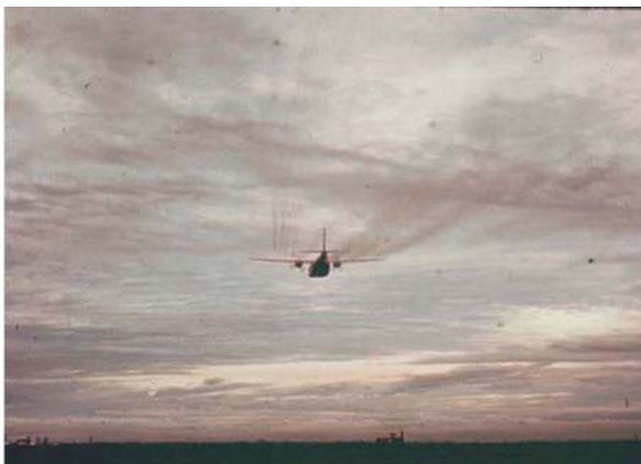
Fig. 6.2 C-123B RANCH HAND aircraft conducting a test and evaluation flight of the MC-1 Defoliant Spray System, Test Area C-52A, Eglin AFB, Florida, 1963 (Photograph courtesy of the AFATL, Eglin AFB, Florida)
