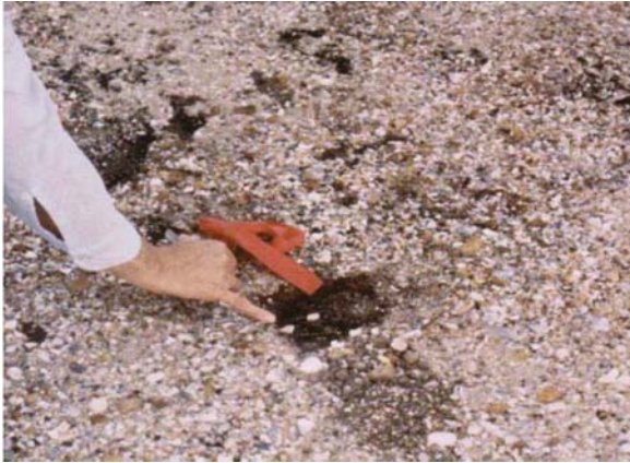
Fig. 7.8 A photograph of a sampling site for herbicide residue from the former Herbicide Orange Storage Site at NCBC in July 1977. Note that the oyster shells were removed before the soil sample was obtained. The sample was collected 15 cm from a numbered metal stake (Photograph courtesy of A.L. Young)
