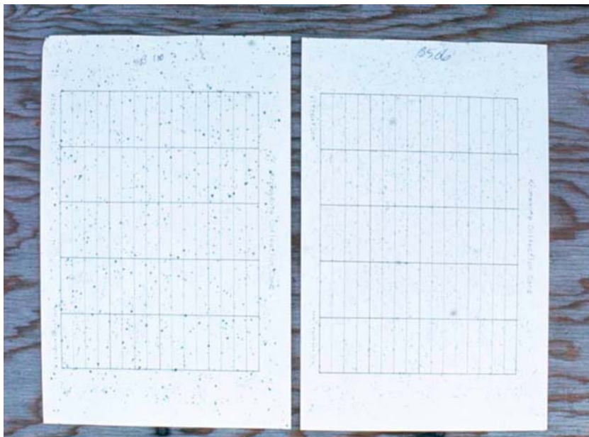
Fig. 6.8 Beginning in May 1968, 550 sampling arrays (two in-wind lines and four cross-wind lines) consisting of glass plates and Kromekote Cards (above) provided physical collection of test materials in droplet forms, Test Area C-52A, Eglin AFB, Florida (Photograph courtesy of A.L. Young)
