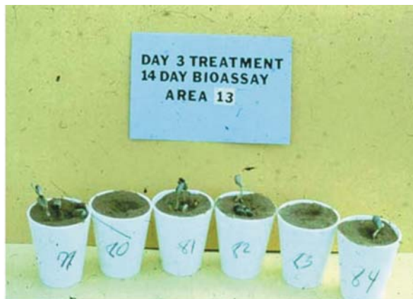
Fig. 6.20 Soybean bioassay of a 90-cm soil core from Site C-9 divided into 15-cm increments ( left to right ) showing positive response to herbicide residues, April 1970, Test Area C-52A, Eglin AFB, Florida (Photograph courtesy of A.L. Young)
