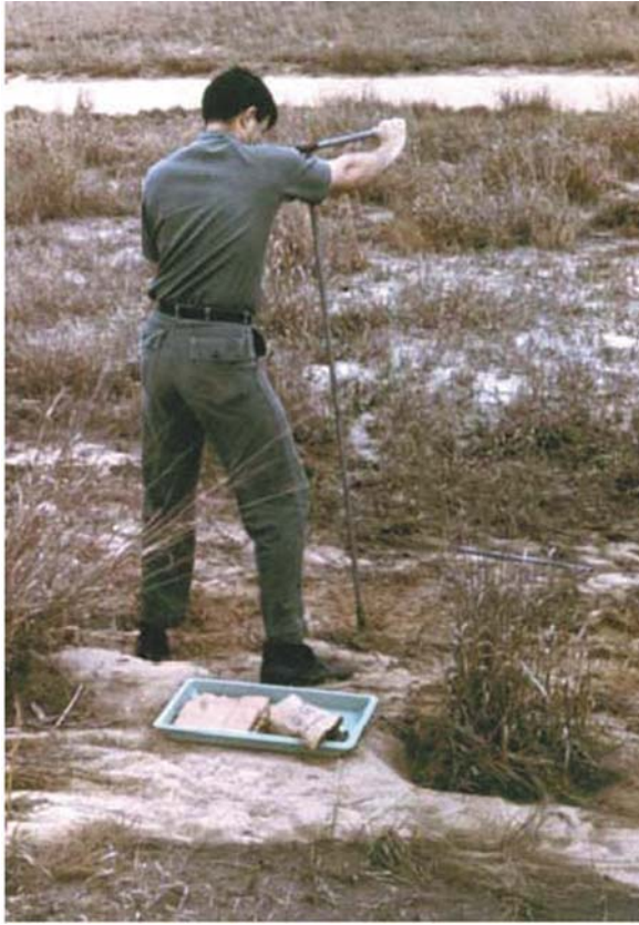
Fig. 6.19 AFATL personnel using a hand soil-coring tool to collect 90-cm cores for herbicide residue study of Test Area C-52-A, Eglin AFB, April 1970 (Photograph courtesy of A.L. Young)
