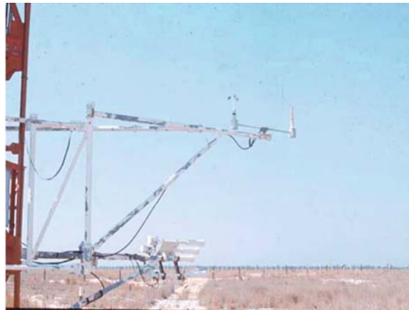
Fig. 6.6 Sampling array for wind, temperature, and droplet dispersal data on the 90-m tower in the center of Test Area C-52, Eglin AFB, Florida, 1969 (Photograph courtesy of A.L. Young)
