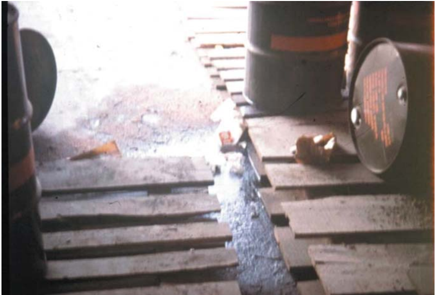
Fig. 3.10 Out of every 10,000 drums of herbicide shipped to Vietnam, about 10 of them (0.1%) were received in a damaged or defective state. Leakage from these drums contaminated the docks and the semi-trailers used to haul them to the RANCH HAND bases (Photograph courtesy of Air Force Logistics Command, Kelly AFB, Texas)
