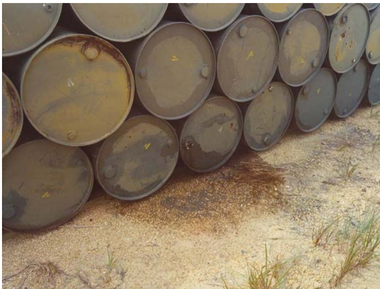
Fig. 7.4 A photograph of a leaking drum in June 1975 within the NCBC Herbicide Orange Inventory (Photograph courtesy of AFLC, Kelly AFB, Texas)
