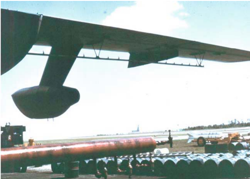
Fig. 6.11 A wing defoliation spray boom mounted on the UC-123 K aircraft at Hardstand 7 in 1969; note drums of Agent White and the Eglin AFB Airdrome in the background (Photograph courtesy of AFATL, Eglin AFB, Florida)
