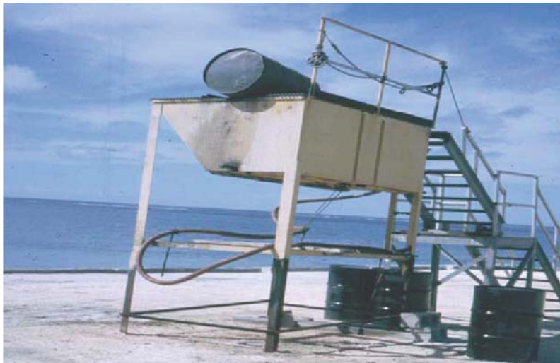
Fig. 4.18 De-drum/Re-drum Facility at Johnston Island, October 1973; approximately 10,000 drums were required to be re-drummed during the years from 1972 through mid-1977 (Photograph courtesy of USAF Occupational and Environmental Health Laboratory, Brooks AFB, Texas)
