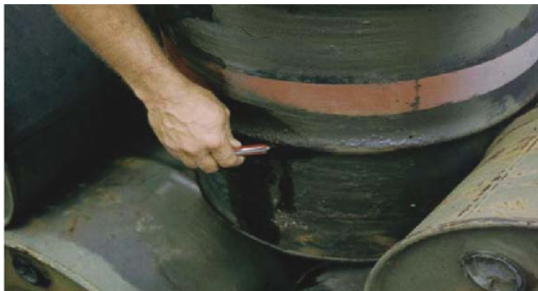
Fig. 4.17 A leaking drum of Agent Orange, 1974 at NCBC, Gulfport, MS. The leak occurred on the “rib” of the drum on the underneath side (toward the ground); A policy was implemented to periodically rotate the drums, thus preventing or minimizing this type of leak (Photograph courtesy of A.L. Young)
