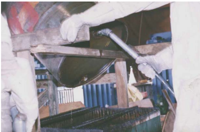
Fig. 4.19 De-drumming and rinsing operation of an Agent Orange drum at Naval Construction Battalion Center, Gulfport, MS, April 1975; a full-time crew was required to maintain oversight of the inventories at NCBC and Johnston Island (Photograph courtesy of AFLC, Kelly AFB, Texas)
