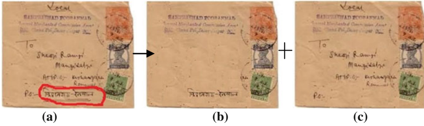
Fig. 1 An example showing the script identification, where a a bi-script sample is expected to separate b Devanagari and c English script
