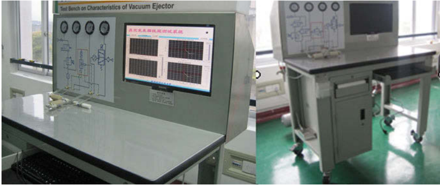
Fig. 10.1 Test benches on characteristics of vacuum ejector and vacuum regulator
