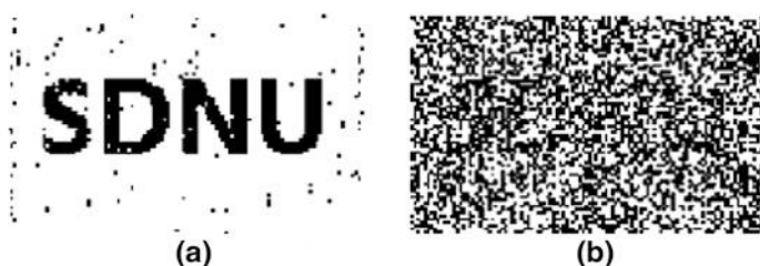
Fig. 107.9 The extracted watermark from MPEG-2 compression attack ( NC = 0.9658, 0.1532 ). a Uncompressed; b compressed
