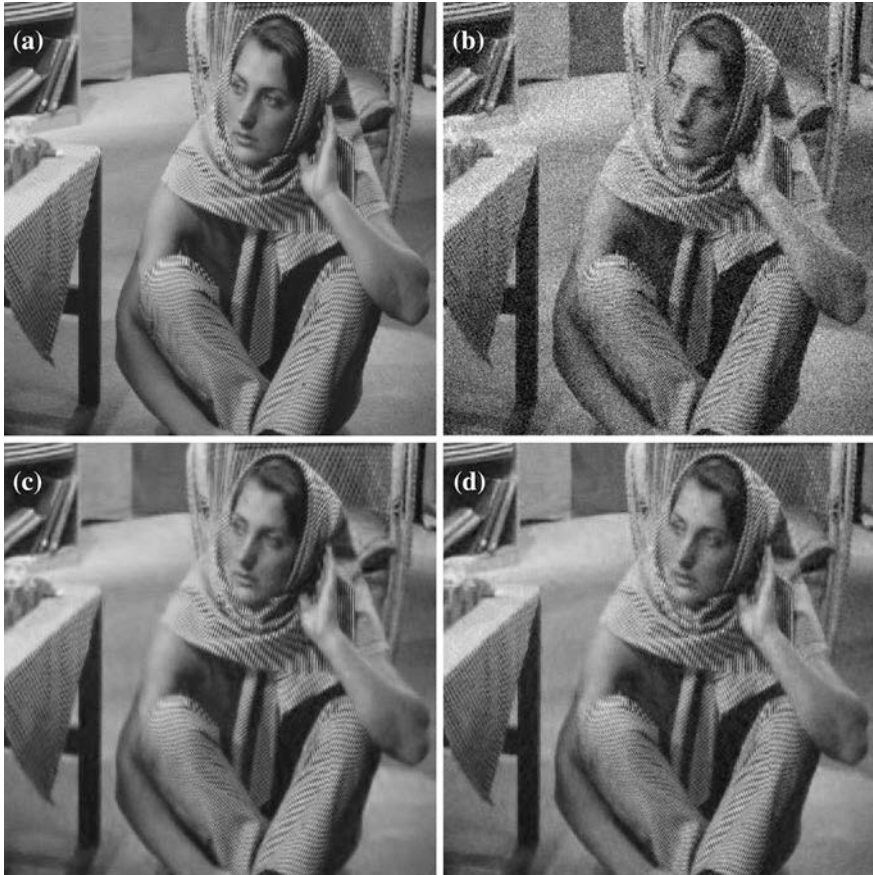
Fig. 35.3 Visual comparison of various denoising method on test image Barbara (at noise level 20). a Original; b noisy image, PSNR = 22.10 dB; c Wavelet-LapMix, PSNR = 29.90 dB; d shearlet-LapMix, PSNR = 30.77 dB
