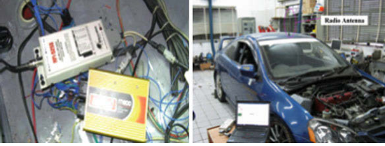
Fig. 53.3 In-car radio transmitter and the location of the radio antenna
