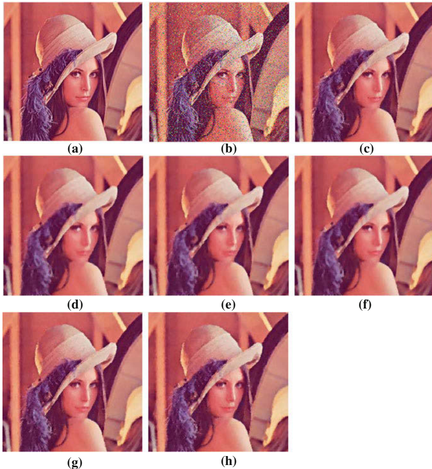
Fig. 96.2 Original Lena image, impulsive noise ( p_v = 0.1 ) image and filtered outputs. a Original Lena image (24-Bit, 256 \times 256 ); b Noise image; c PCNN-DDF; d VMF; e BVDF; f DDF; g Rank SVMF; h Mean SVMF
