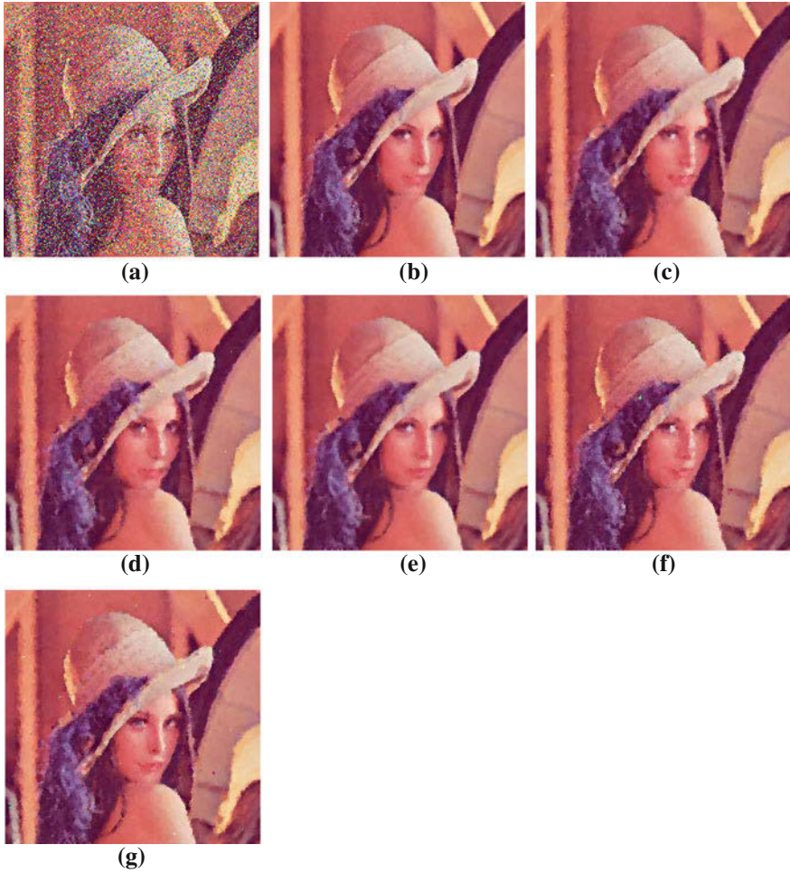
Fig. 96.3 Impulsive noise ( p_n = 0.3 ) image and filtered outputs. a Noise image; b PCNN-DDF; c VMF; d BVDF; e DDF; f Rank SVMF; g Mean SVMF
