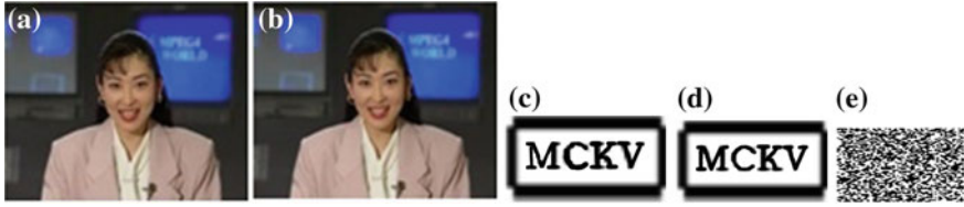
Fig. 11.1 a Original frame of Akiyo. b Watermarked frame of Akiyo. c Original watermark image ( 50 \times 25 ). d Extracted watermark ( 50 \times 25 ) from all watermarked video with NCC = 1 . e Extracted watermark using fake key. ( P, M, \varepsilon ) above each image represents the PSNR (in dB), MSSIM and security values of the watermarked video frame. ( P : 43.99, M : 0.98, \varepsilon = 0.0011 )
