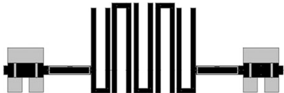
Fig. 3.4a Modified hairpin BPF with DGS and DMS in feed line
