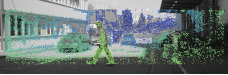
Fig. 12.1 Color coded stereo measurement in a typical road environment
