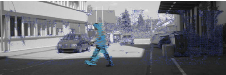
Fig. 12.2 Flow measurement in the same scene like Fig. 12.1. The warmer the color the longer the flow vector
