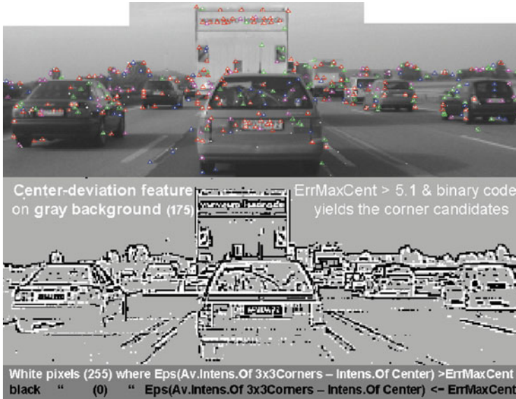
Fig. 11.4 Highway scene with candidates for corner features (white and black, bottom) selected by the “center-deviation test” using the average of the four corner pixels of the 3 \times 3 mask (Fig. 11.3, bottom, \sim 14\% ). The orthogonal curvature cross-test reduces this number to \sim 3.5\% , the rotated tests to \sim 0.8\% . After fusion of \sim 260 local candidates, about 600 corner features are obtained (top, region of special interest); they are marked by triangles
