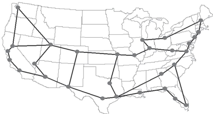
Fig. 10.2 Reference Network 3. With a relatively low nodal density, increasing the reach from 600 to 1,500 km can provide a cost benefit even in a network based on O-E-O technology
