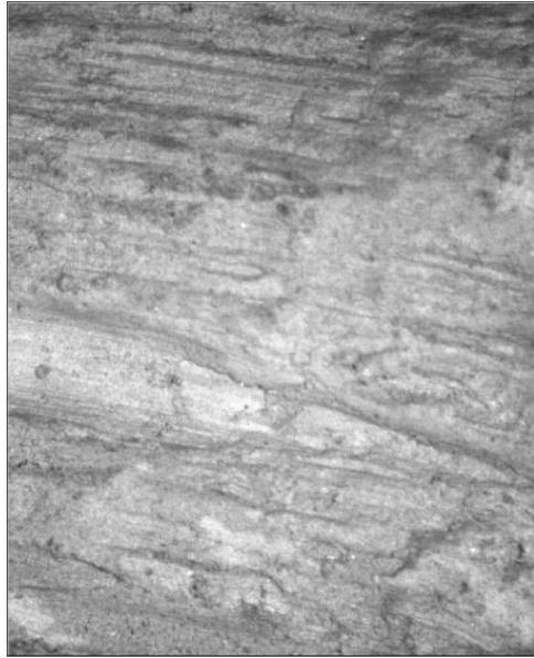
Figure 5.15 Common view from shear surfaces of XT set sheared at slow rate.
