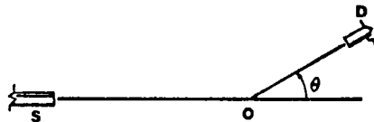
FIG. 1. Schematic set-up of a scattering measurement. Radiation (light) source (S) illuminates scatterer (O), and detector (D) records scattered intensity at angle ( \theta ) as it rotates about (O) at a fixed distance from it.
