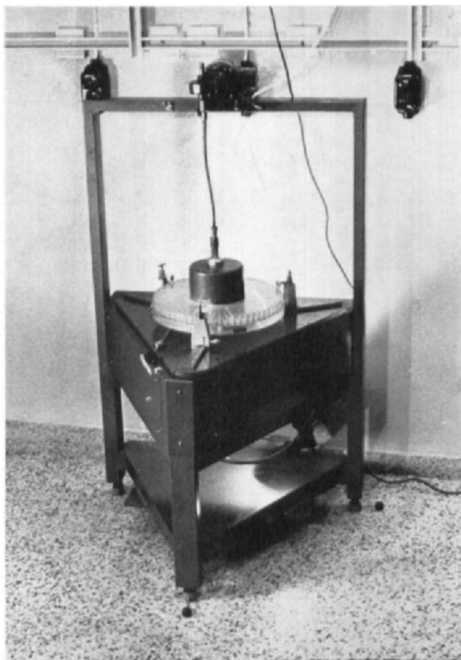
FIG. 15. Automatic version of the thin-layer counter-current distribution apparatus.
