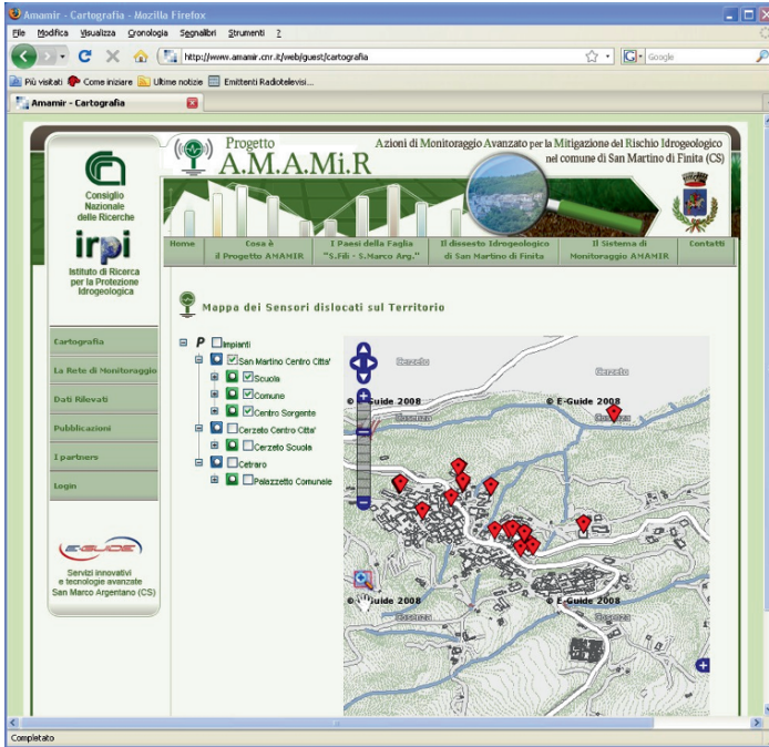
Figure 2. WebGIS portal for reading remote sensors data in real time ( www.amamir.cnr.it ).
