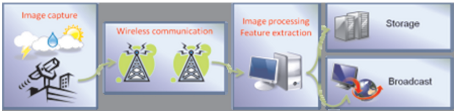
Figure 3. Skeye system architecture.
