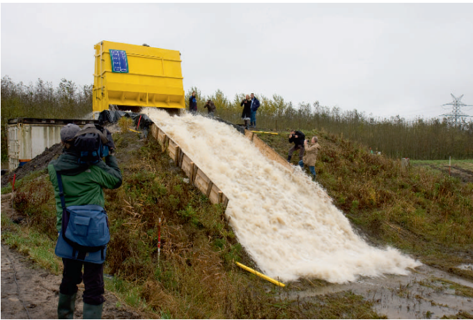
Figure 1. Small scale wave overtopping experiment using a wave simulator.
