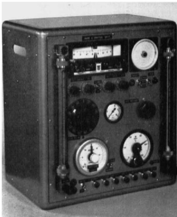
FIG. 3. Control box. The upper third of the front panel houses the instruments for automatic pH control (an EIL Model 91A pH Indicator-Controller and an Elmes 12 Cyclogram Recorder, with associated switches); the lower third houses the antifoam timer (left) and temperature controller (right); the centre area locates the air-flow controllers (each side), air-pressure regulator (right) and Variac auto-transformer (left). A main fuse, indicator light and series of switches are positioned along the bottom of the panel.
