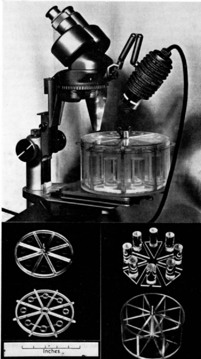
FIG. 12. The Jarvis chamber for hygroscopic studies, with details of the component parts. (Reproduced by courtesy W. R. Jarvis.)
