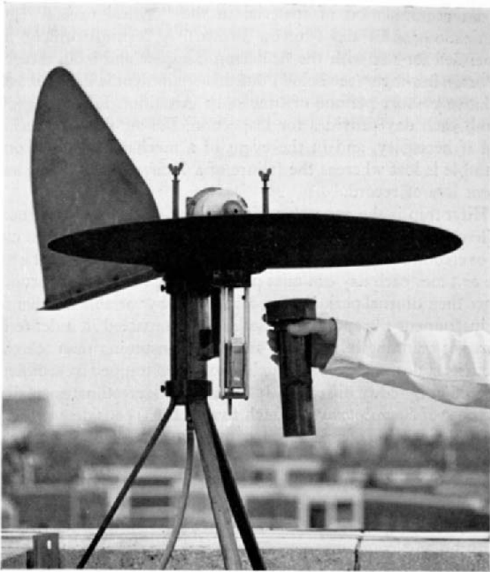
FIG 4. (b) Body of trap with sampling aperture removed to show slide.
