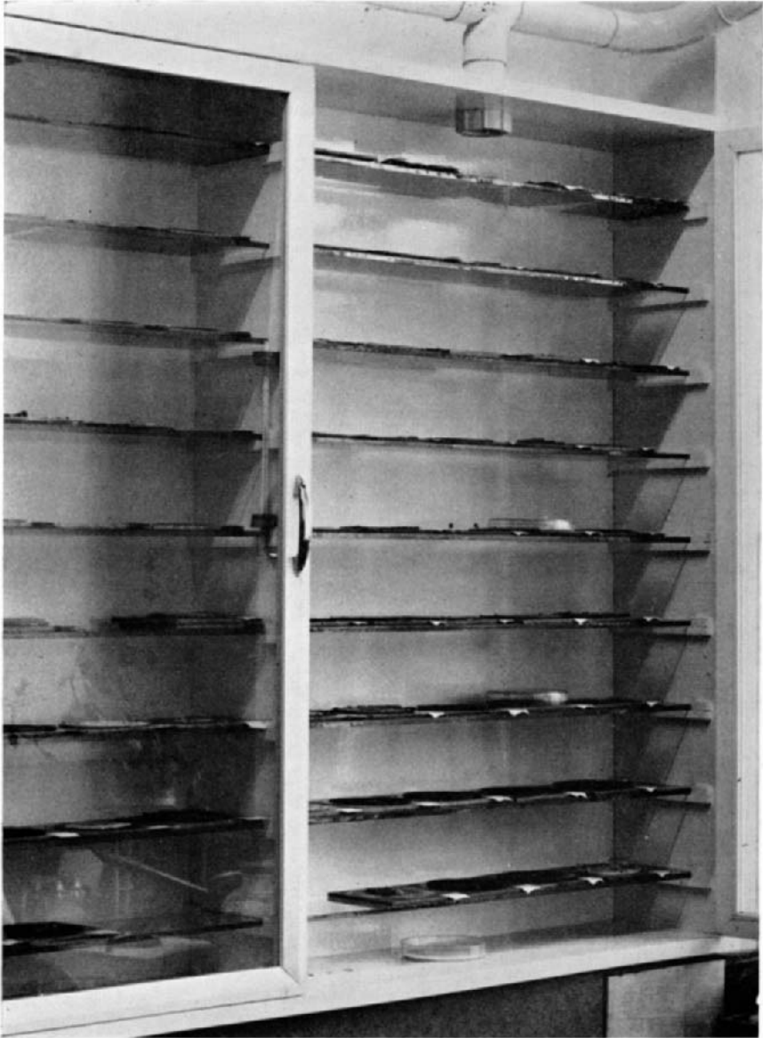
FIG. 6. Preparation of dried agar cultures. Drying cultures in a drying cupboard. This gives more controlled drying and prevents dispersal of the spores into the laboratory. (Photograph by D. W. Fry.)
