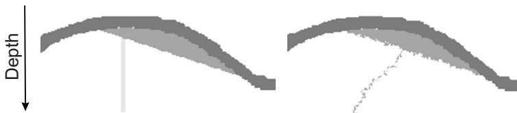
Fig. 6.54. Invasion percolation pathways below an accumulation according to Fig. 6.53. The figures are calculated without and with heterogeneities, respectively
