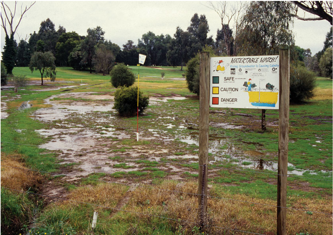
Fig. 3.14 A flagpole floating in a shallow well is an indicator of water table height and thus potential for salt damage to soil. If the red part of the flag is showing above the soil surface, then the water table is within a meter of the surface and thus there is danger of salt accumulation on the ground surface. Recent irrigation has left the ground surface wet, but the poor vegetation cover indicates that this area has a high salt content. Shepparton, Australia
