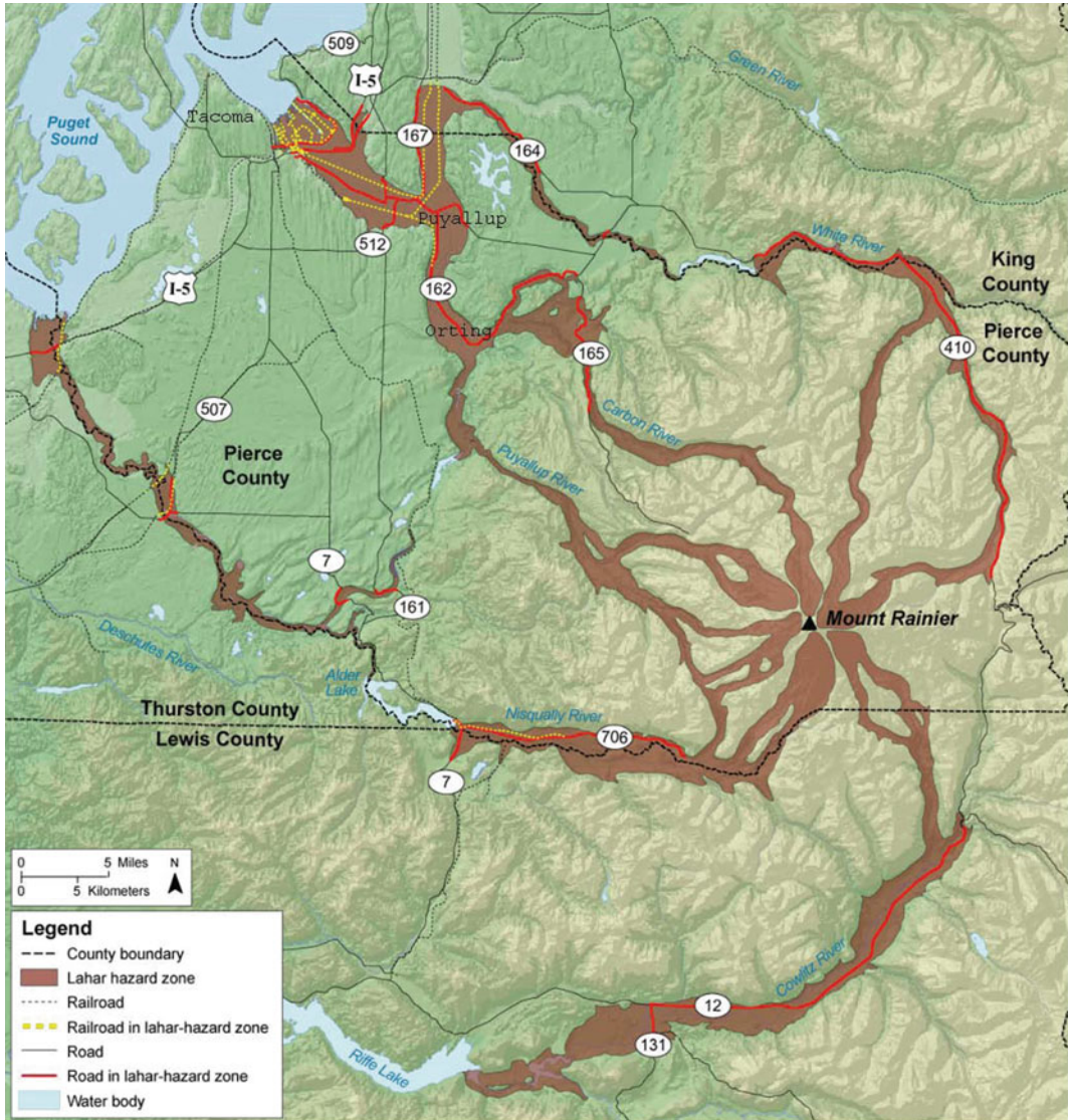
Fig. 7.21 Hazard map of potential lahar flows from Mount Rainier to Puget Sound in the United States. Lahars tend to flow down river valleys but can spread out across the landscape. They have potential to damage low-lying houses and infrastructure such as roads and bridges (Map from United States Geological Survey)
