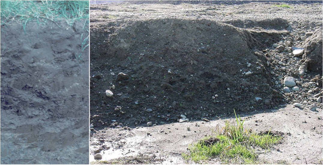
Fig. 8.26 Changes in the soil environment due to urban development. Left: a valley bottom soil from Western Washington state prior to urban development. Right: the natural soil of this urban valley has been completely replaced with new material that is a more suitable substrate for construction
