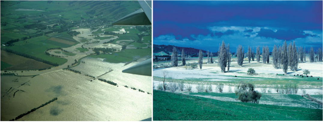
Fig. 3.5 River floodplains are subject to periodic inundation. Left: Floodwaters overflow a river stopbank to inundate an area of farmland in New Zealand. Here the river stopbank is designed to be overtopped so the excess flood waters safely flow out into an area that is free of houses, thus protecting a town further downstream from flooding. Right: mud (silt and clay) deposited by a major flood can be seen covering the floodplain of the Waipaoa River in New Zealand. The river waters, though having now receded into the river channel, are still a pale color due to the load of mud they are carrying
