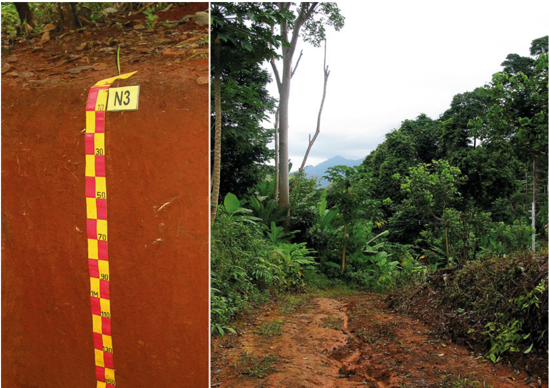
Fig. 4.20 A deep, highly weathered, old tropical forest soil in Thailand. This soil is rich in iron and aluminum oxides. Weatherable minerals have been broken down and soluble nutrients have leached. The iron oxides give this soil its characteristic bright orange-red color
