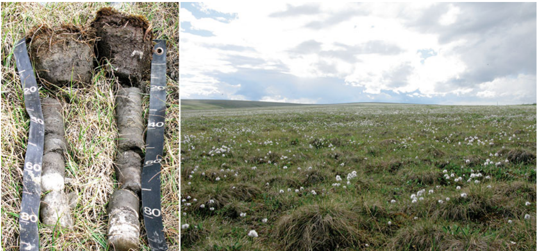
Fig. 3.22 Arctic peat soils on the North Slope of Alaska. Left: while the near surface soil is thawed in summer and can be cut with a spade, the deeper soil is frozen solid, so a corer was used to extract it. The white-colored parts of the core are ice. Right: the North Slope of Alaska, near the Arctic Ocean, is a vast swampy tundra plain. There is a high water table and the area is interspersed with many small lakes in summer and covered in snow in winter
