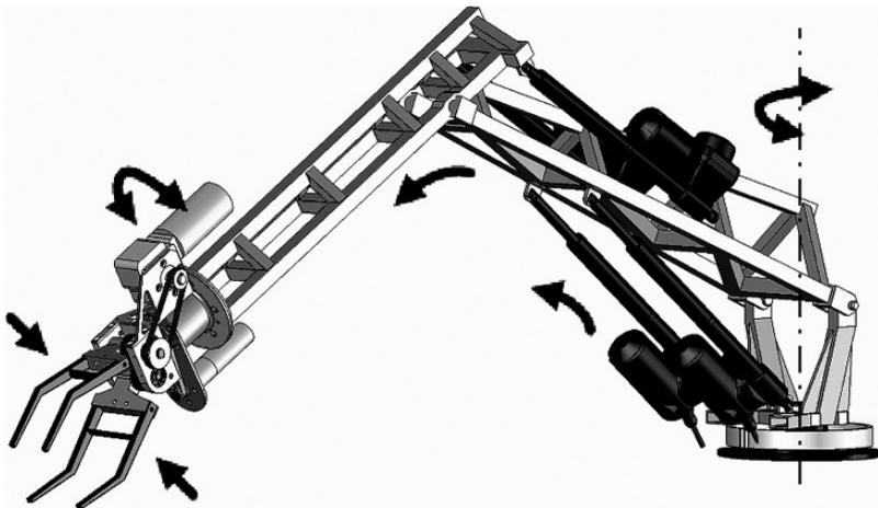
FIGURE 16.1. Sketch of a robotic arm with 5 degrees of freedom.
