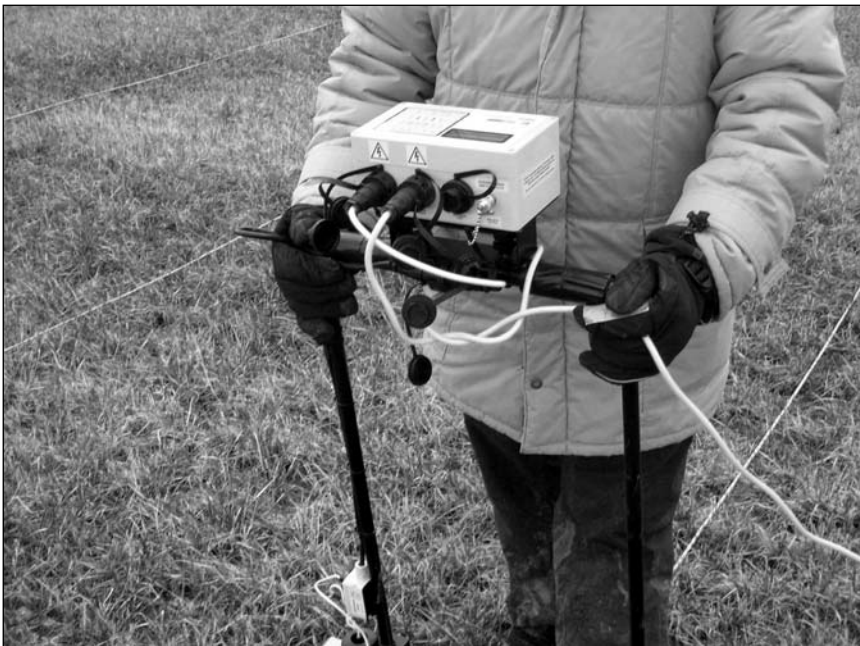
Figure 5.10 Connect the frame probe and remote probe cables to the meter. Make sure there is a loop in the remote probe cable, so that takes the strain, not the connector.
