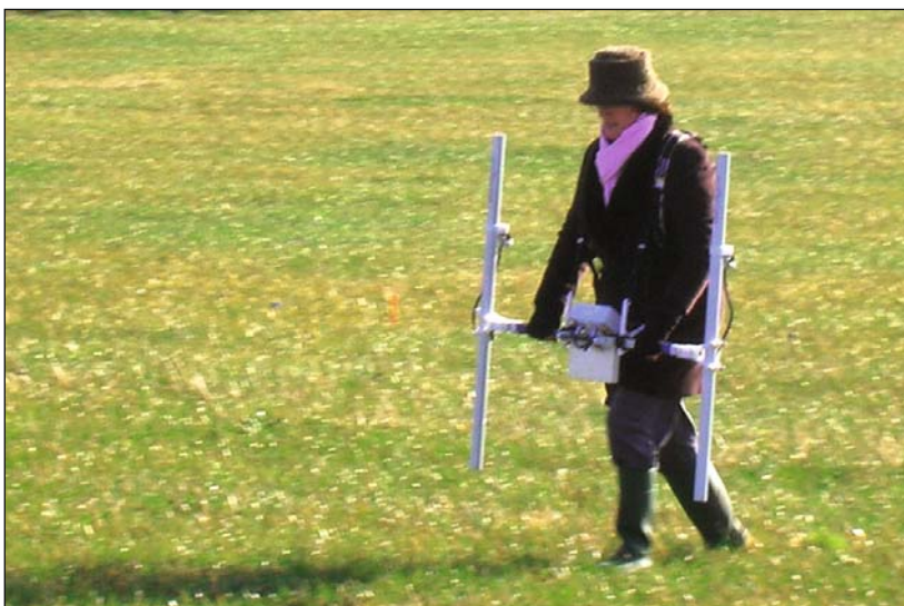
Plate 4 Surveying using a Bartington 601/2 dual gradiometer. Each tube is an individual gradiometer, so this device can survey two lines at once.
