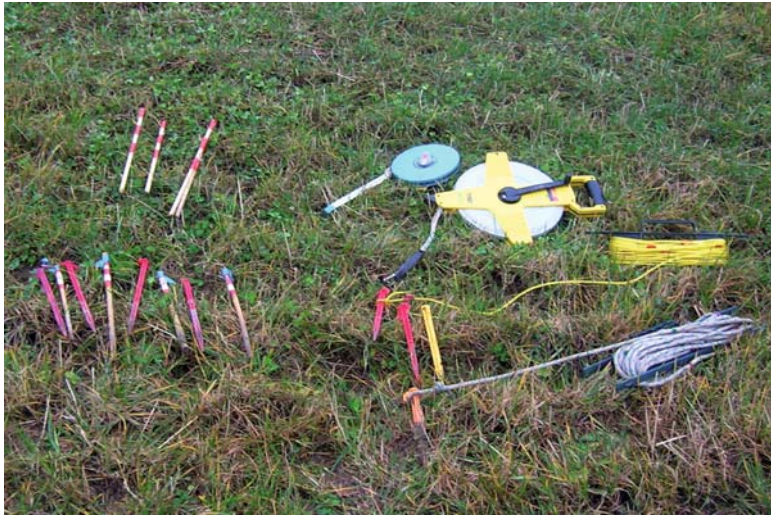
Plate 13 Ancillary components you need: (top left) grid corner posts; (bottom left) flags and pegs (30cm pegs); (top right), measuring tapes, 30m and 100m shown here; (bottom right), grid lines made from washing line, with pegs (20cm) and wound on a former, and a rope walking line, wound on a former.
