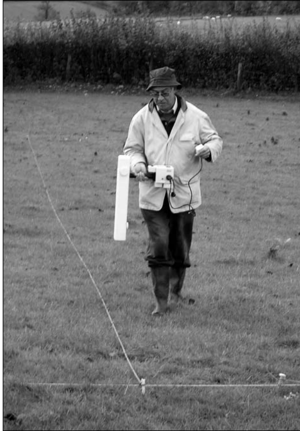
Figure 3.11 Surveying using a Geoscan FM256 gradiometer. Note the use of a walking string as a guide.
