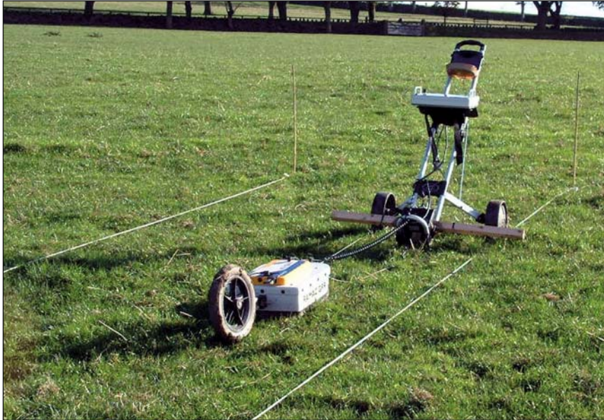
Plate 7 A typical radar set ready for use. The controls are on the buggy, with the antenna towed behind, and the wheel behind that measures distance.
