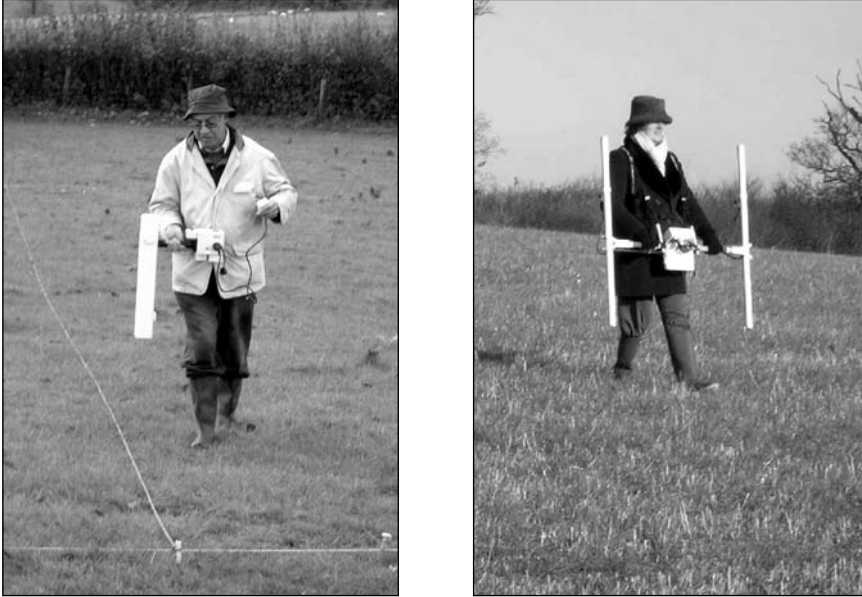
Figure 1.1 Fluxgate magnetometers. The two shown here look very different, but are similar in principle, with a detector at either end of a long tube, each measuring magnetic effects at a different height from the ground.
