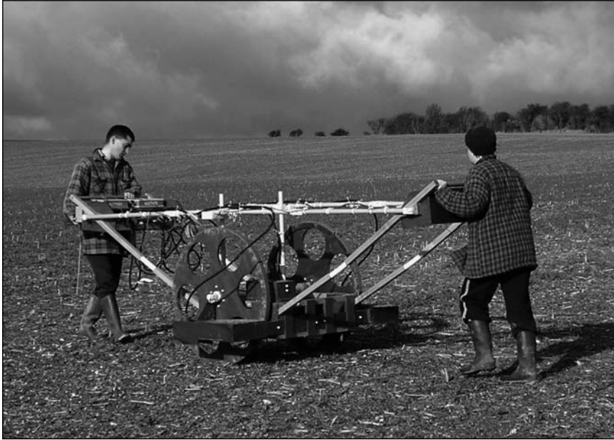
Figure 3.7 The ‘wobbly cart’ belonging to English Heritage. It is designed to carry caesium magnetometers in a non-magnetic, suspended environment.
