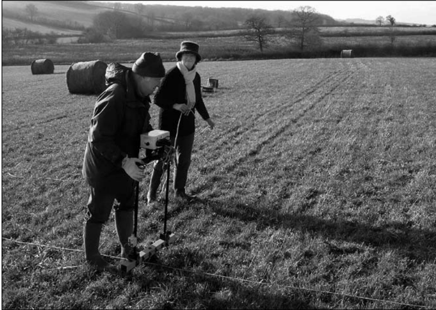
Figure 3.4 Surveying with twin probe resistance measurement. The frame holds a voltage and a current probe, as well as the control box. A cable connects to the remote probes.
