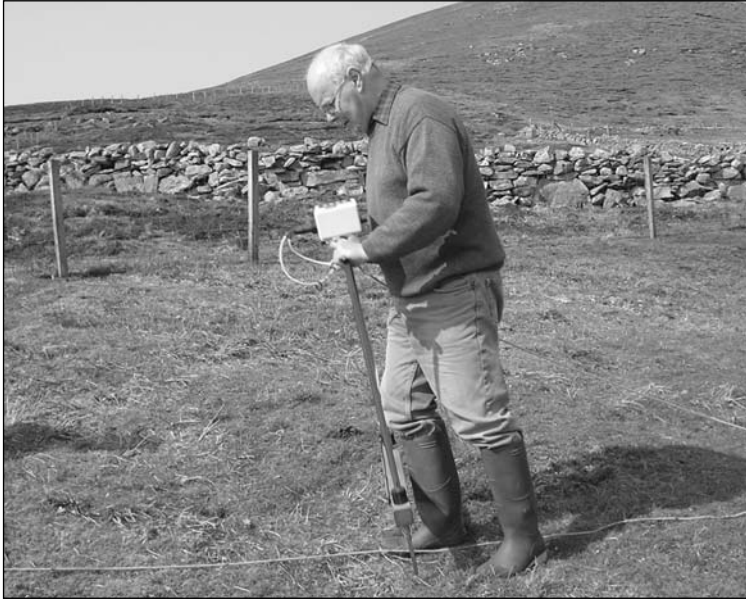
Figure 1.2 Resistance measurement. The frame has a voltage probe and current probe, and there are also remote voltage and current probes at the end of a long cable. Dividing voltage by current gives the resistance.
