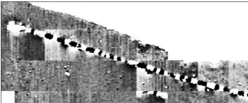
Figure 3.10 Stripy pattern caused by a metal water pipe.
