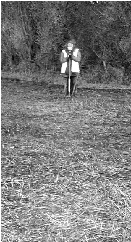
Figure 3.21 The target is on the pole held steady at the point to be measured.
