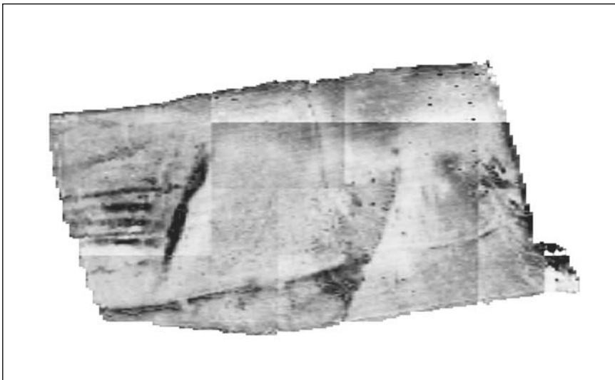
Figure 4.5 Resistance plot, showing a field with stone drains (left), and a wall which goes to a small house (bottom centre).
