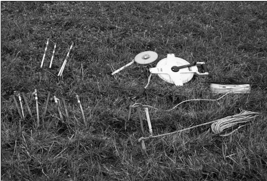
Figure C1 Ancillary components you need: (top left) grid corner posts; (bottom left) flags and pegs (30cm pegs); (top right), measuring tapes, 30m and 100m shown here; (bottom right), grid lines made from washing line, with pegs (20cm) and wound on a former, and a rope walking line, wound on a former.
