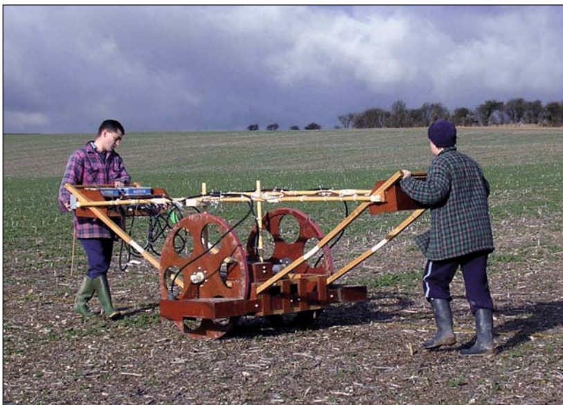
Plate 3 The 'wobbly cart' belonging to English Heritage. It is designed to carry caesium magnetometers in a non-magnetic, suspended environment
