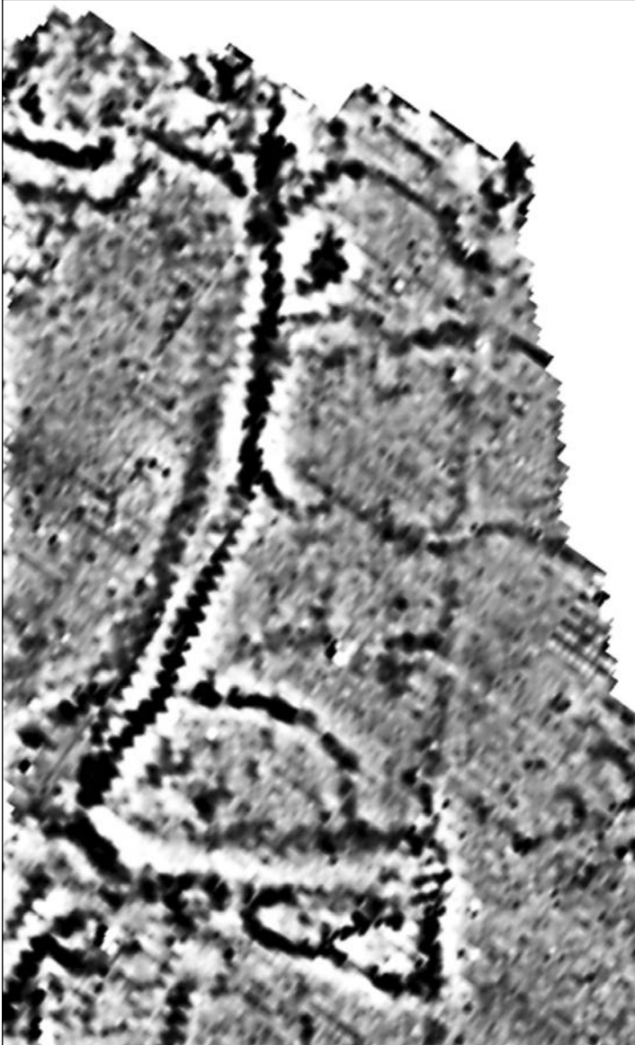
Figure 1.3 Computer output of magnetometer survey. The dark lines represent former ditches in a now-featureless field.
