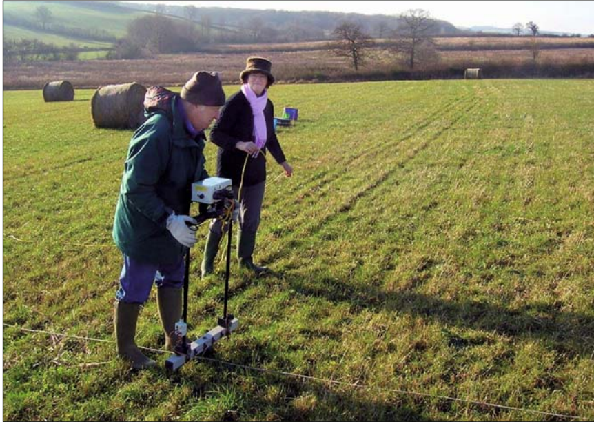
Plate 1 Surveying with twin probe resistance measurement. The frame holds a voltage and a current probe, as well as the control box. A cable connects to the remote probes.
