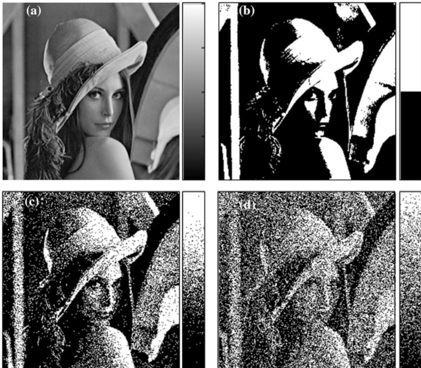
Fig. 6.2 (a) Grey version of Lena standard image; (b) Black-and-white version of the original image; (c) Black-and-white version of a dithered image with moderate noise; (d) Black-and-white version of a dithered image with large noise. (based on Ref. [7])
