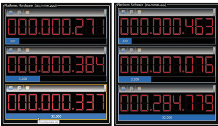
Fig. 3 Comparison of 320, 3200, 32 K comparative searches in hardware (left) versus S/W (right)
